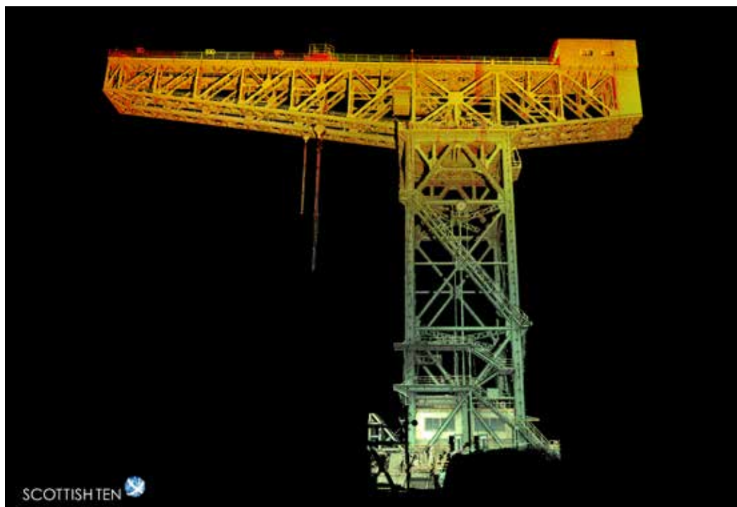
3D point cloud of the Giant Cantilever Crane in Nagasaki, Japan which has been documented by the Scottish Ten project. © Centre for Digital Documentation and Visualisation LLP
