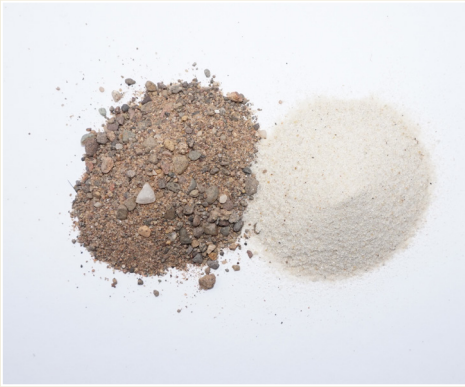
Fig. 3 Well graded sharp sand (left) for backing coats and fine sand (right) for finishing coats.
