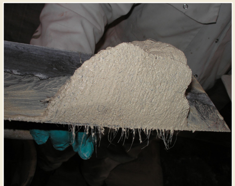
Fig. 5 Hair should be evenly distributed through the mix, appearing as a 'beard' of hairs on the trowel.
