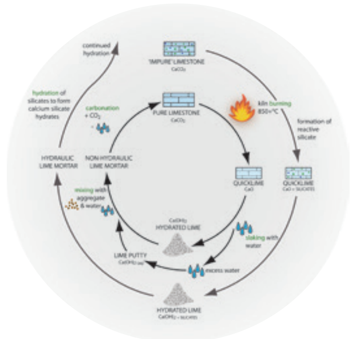
04 Fig. 4 The lime cycle. The cycle is different for non-hydraulic and hydraulic limes due to differences in the composition of the original limestone.
