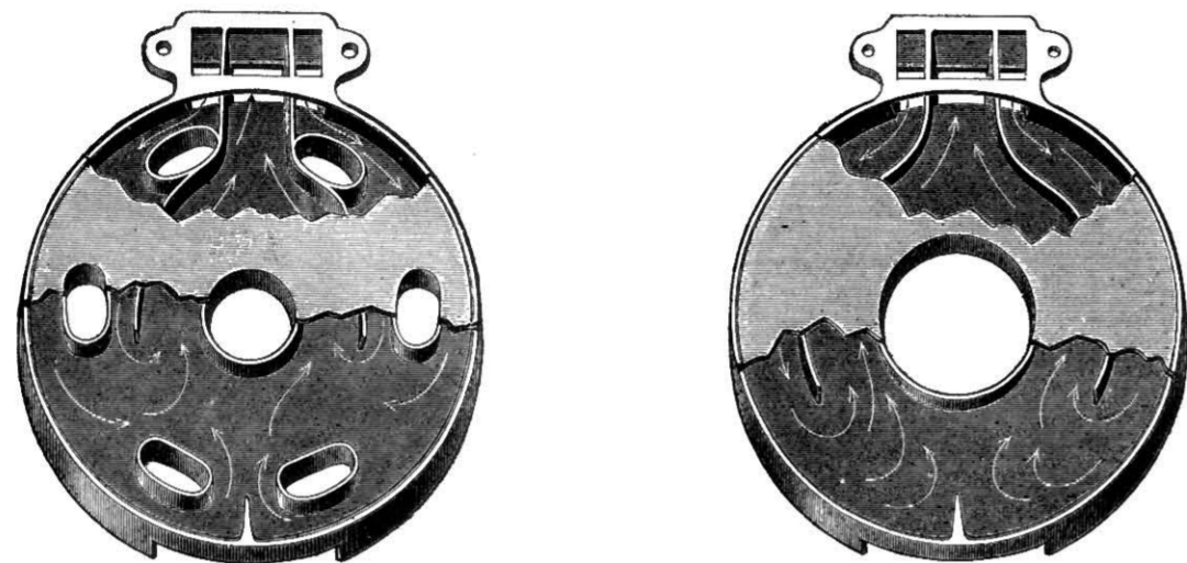
Fig. 511.—View of two Rings of the "Oxford" Boiler, showing circulation of water and back connection.
