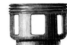
Seating screwed into valve body.
