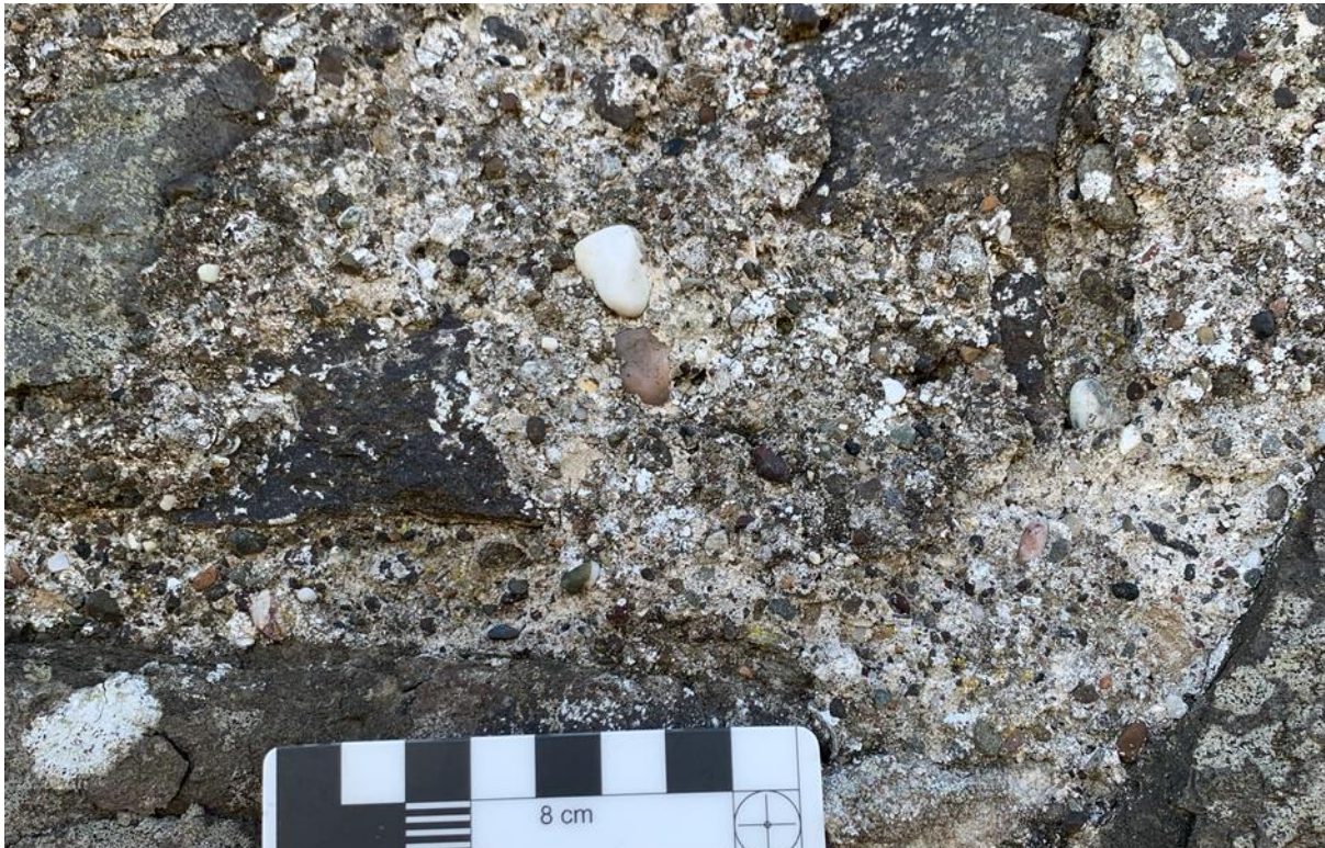
Figure 093.2. Large, rounded aggregates with lime inclusions.
