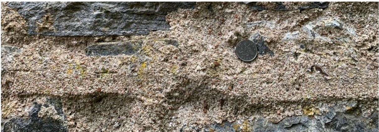
Figure 024.5. Sharp well graded aggregates.
