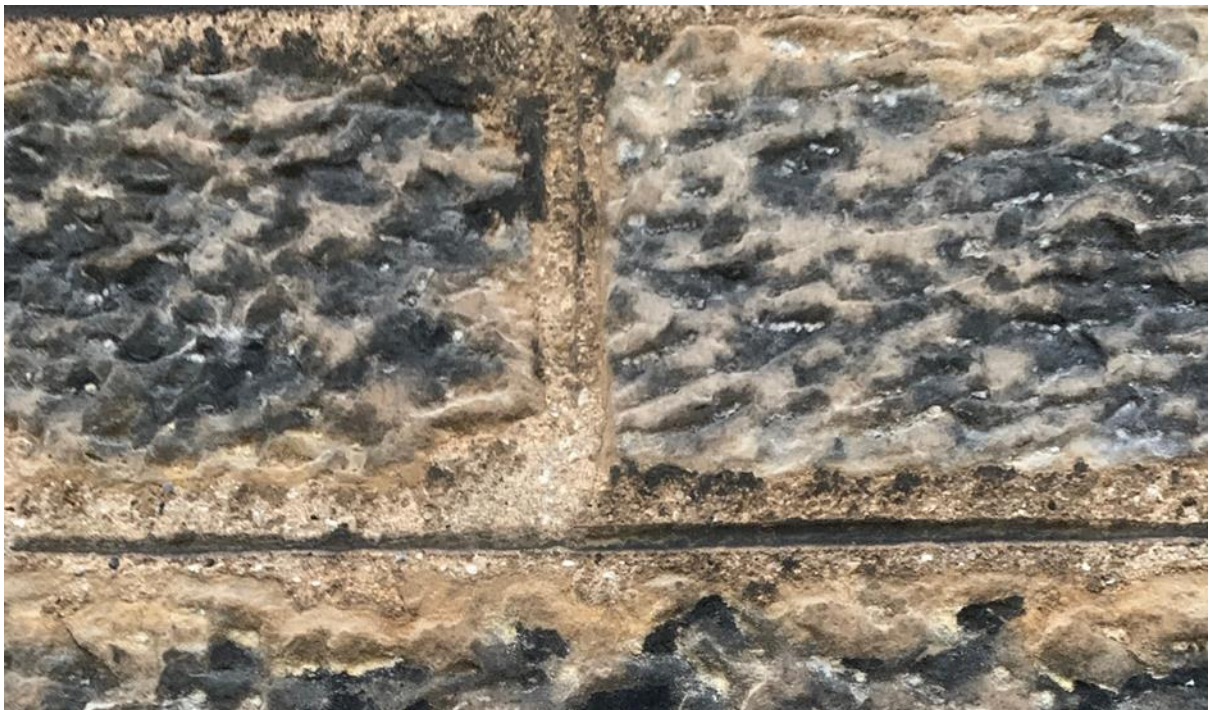
Figure 074.3. Sharp and angular sand with lime inclusions.
