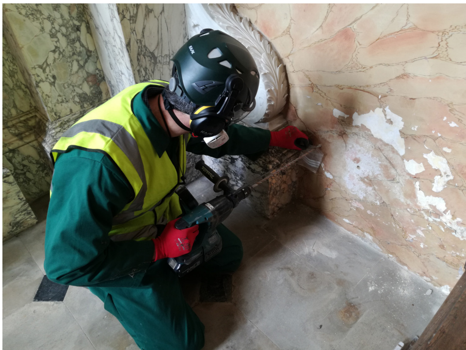
Figure 19 - Powder being collected in a sample bag for gravimetric analysis.
