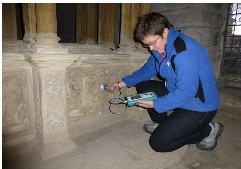
Figure 23 - A microwave sensor being used to determine variations in sub-surface moisture.
