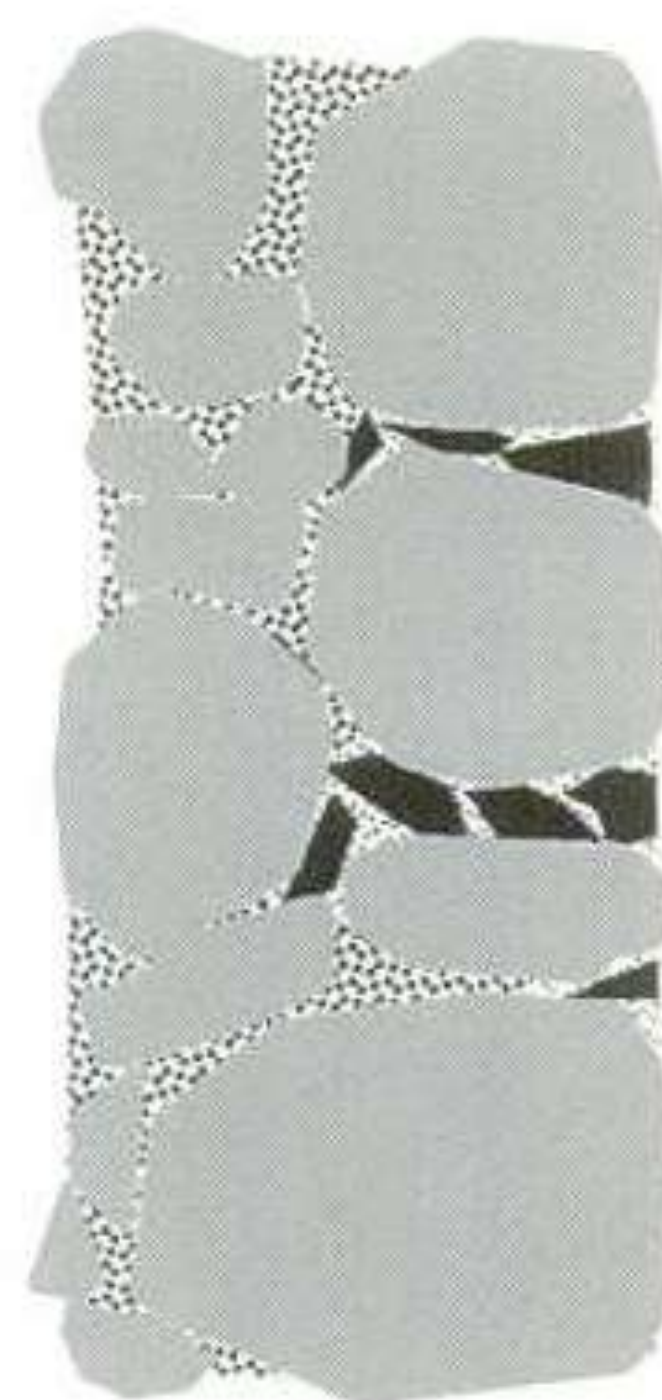
Fig 5 The use of packings and pinning stones
