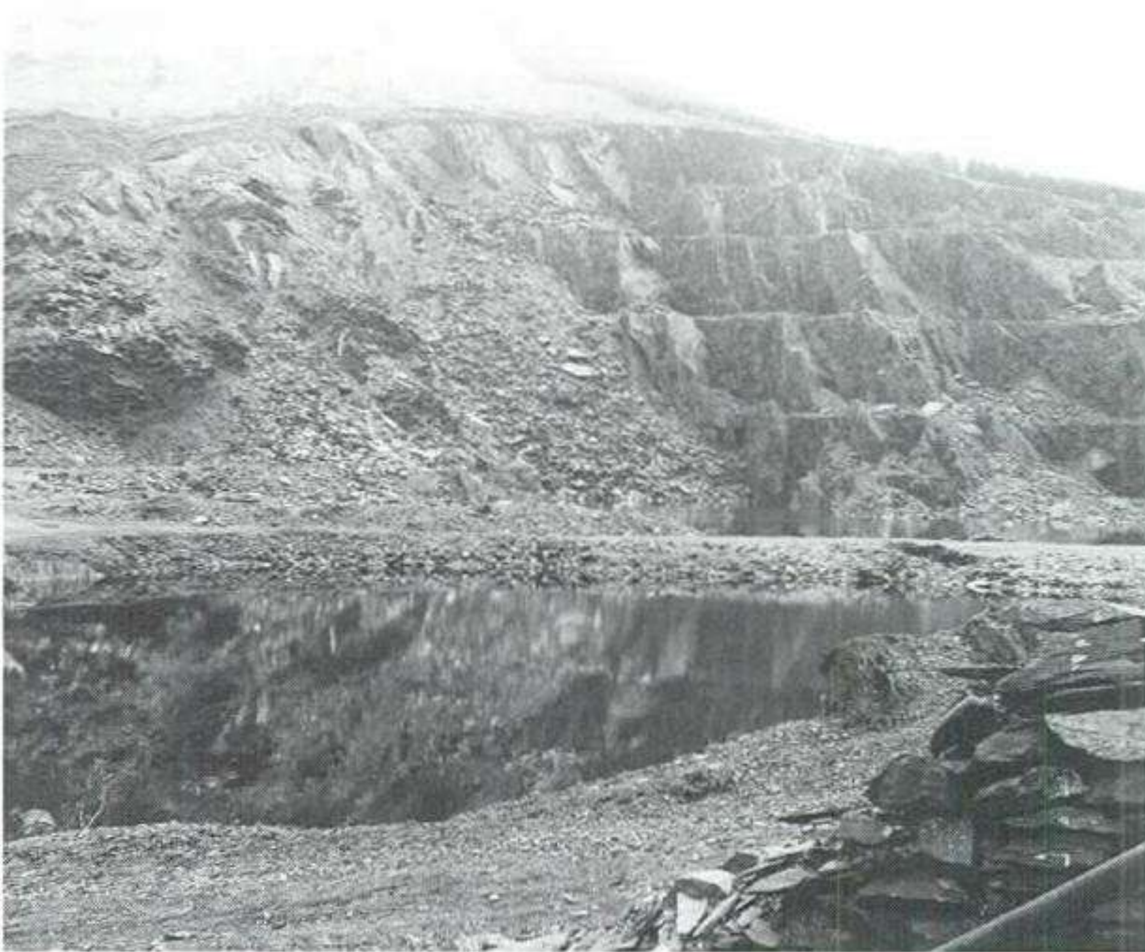
Working faces at East Laroach slate quarry, Ballachulish in 1974. The terraced system of working, though typical of North Wales, was rare in Scotland
