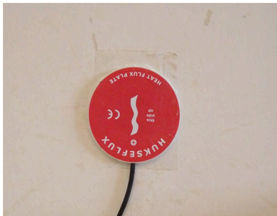
Fig. 1 Heat flux transducer (heat-flow mat) mounted to the wall face
