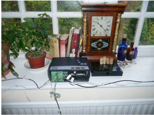
Fig. 3 Grant Squirrel data logger to log data from heat flux transducers and thermocouples
