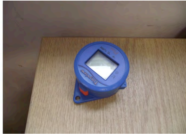
Fig. 4 Stand-alone Tinytag View2 data logger measuring air temperature and relative humidity
