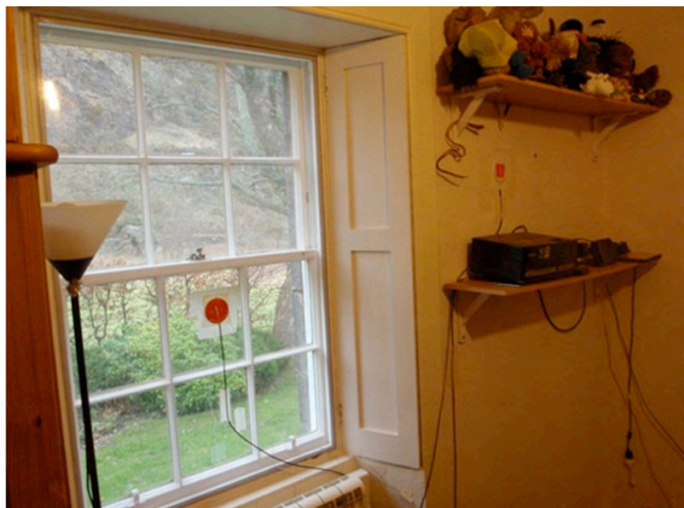
Fig. 12 Heat-flow mats on the window glass and wall
