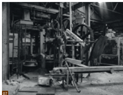
Fig. 7 Machines such as this at Drumpark Brickworks allowed methods such as the stiff plastic process to be used with colliery shale as the raw material (copyright RCAHMS).
