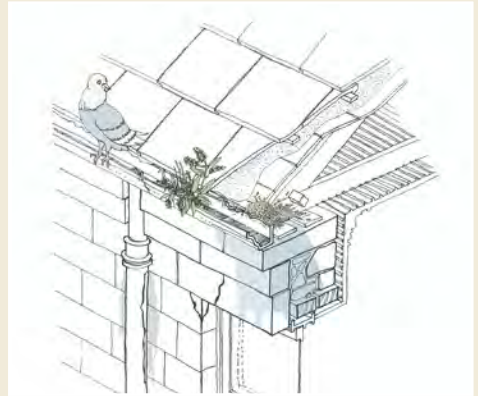
Fig. 3: If your gutters are blocked, rain will run into the inside of your walls leading to rot.
