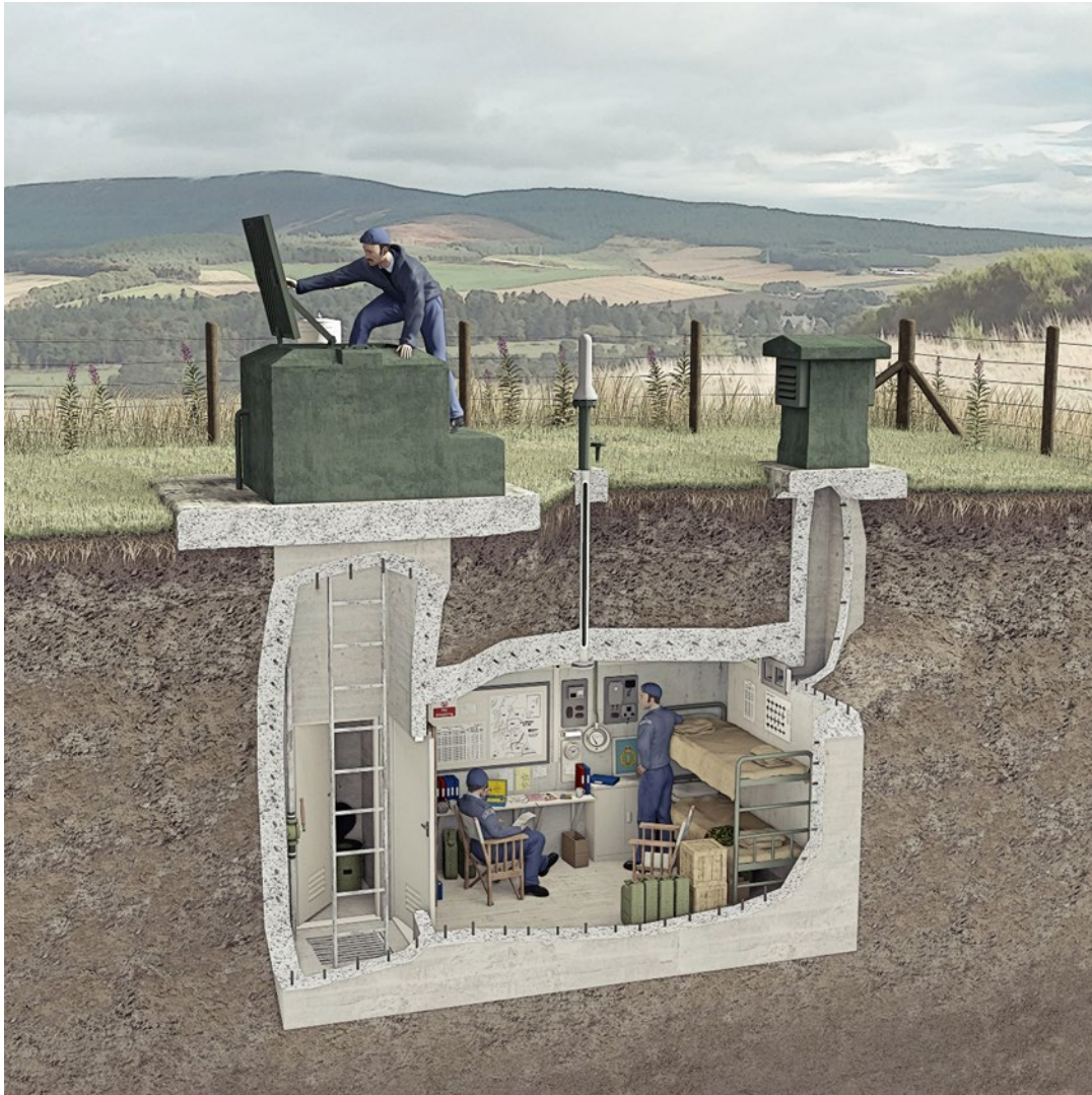
Figure 2: Reconstructed cutaway drawing of Tomnaverie ROC Post showing ROC observers at work. © Crown Copyright HES
