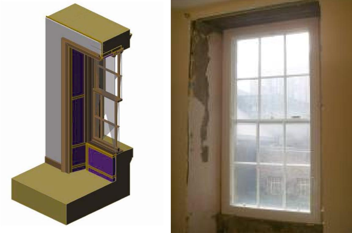
Fig. 13. Diagram and photograph showing insulation locations
