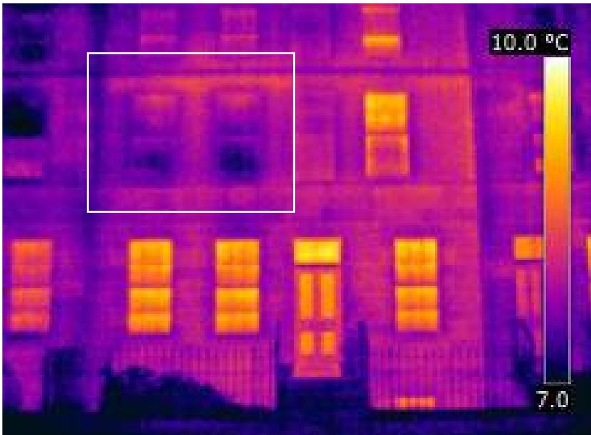
Fig. 34. Thermographic image of property E, showing the improved glazing
