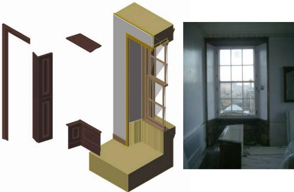
Fig. 20. Diagram and photograph showing downtakings
