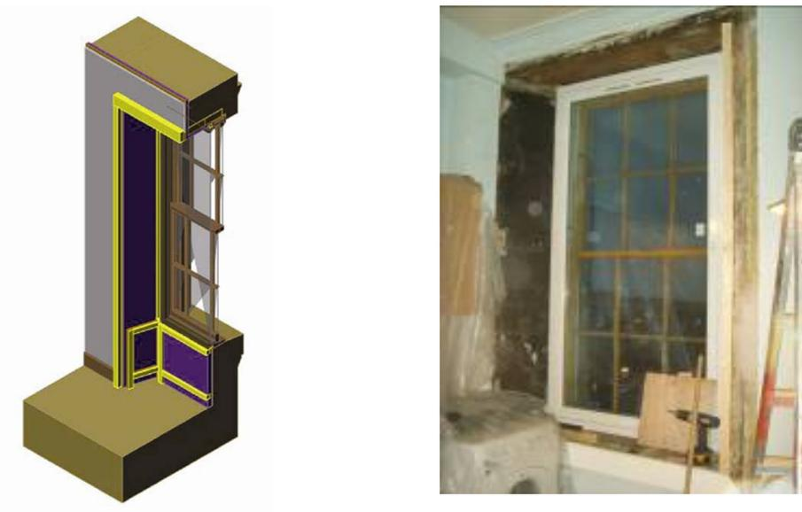
Fig. 26. Diagram showing removal of facings and soffit
