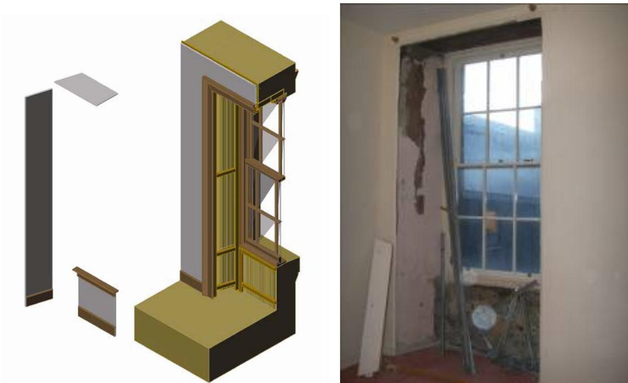
Fig. 12. Diagram and photograph showing downtakings
