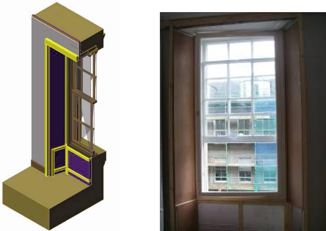
Fig. 31. Diagram and photograph showing insulation work to window opening
