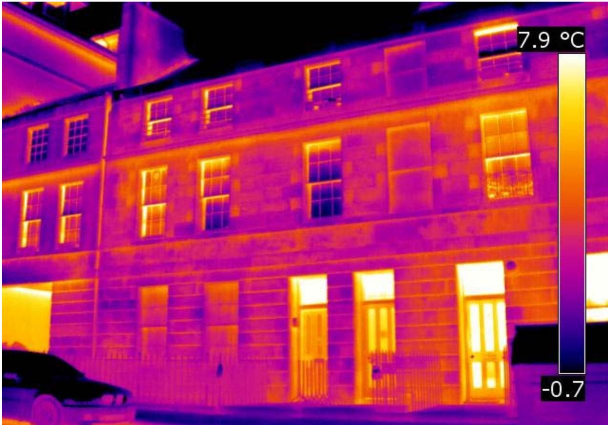
Fig. 35. Thermographic image of 16 Roxburgh Street, showing the thermal improvements to the ground floor windows on the left © Crown copyright (Historic Scotland)
