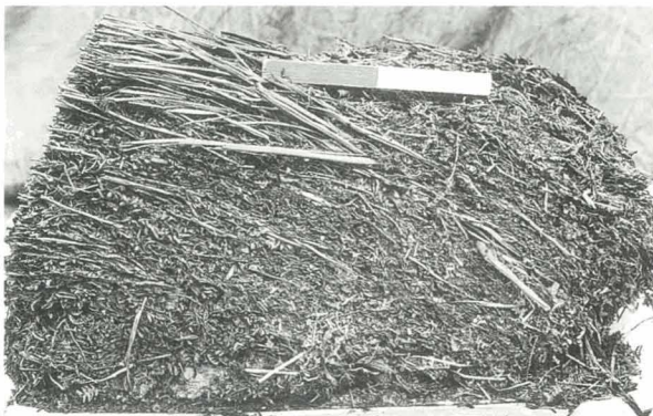
Sections through the thatch block.
