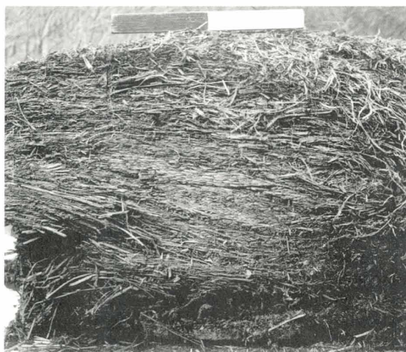
Sections through the thatch block.
