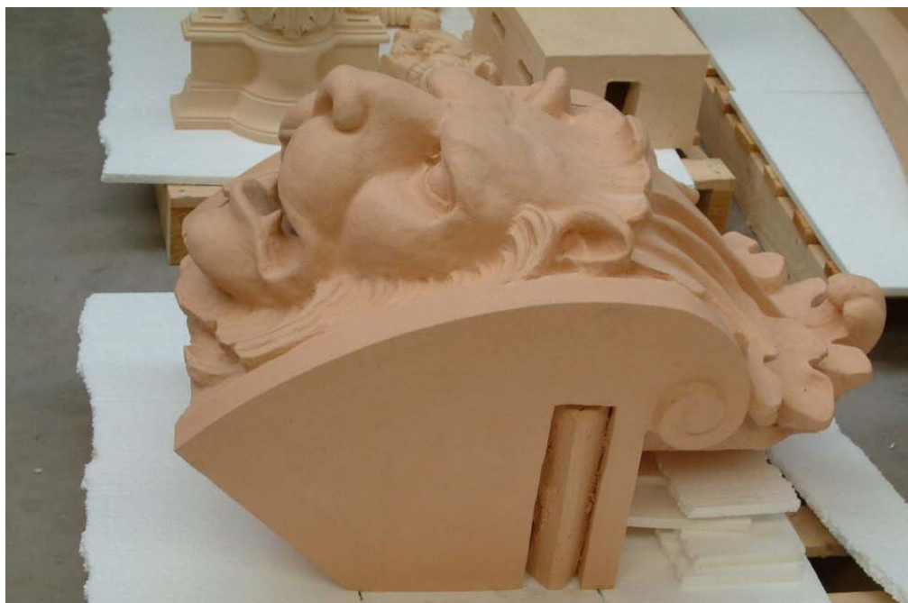
Fig. -9: A replacement terracotta unit manufactured to replace one which had suffered severe deterioration
