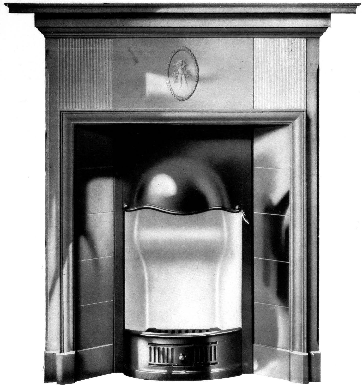
No. 790 TILE MANTEL GRATE, with Single Shelf, Adjustable Cast-iron Canopy, "Douglas" Fire, with Sliding Draught Regulator, W/S Solid Brick Back and Vent Damper. Prepared for Tiles.
