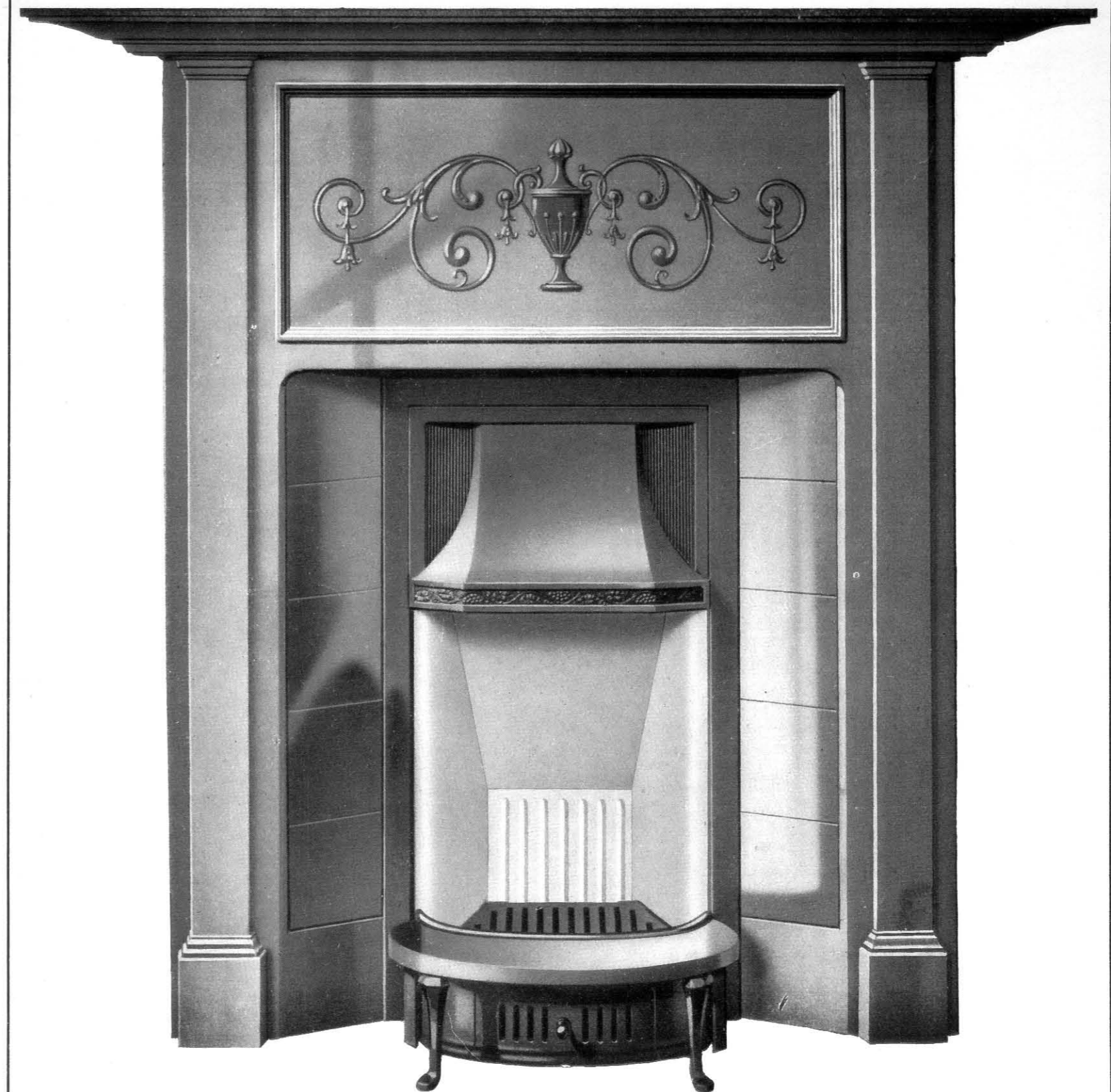
No. 801 TILE MANTEL GRATE, with Double Shelf, Adjustable Cast-iron Canopy, "Vulcan" Fire, with Sliding Draught Regulator, No. 43 Trivet Hob, Brick Back in four pieces. Prepared for Tiles.
