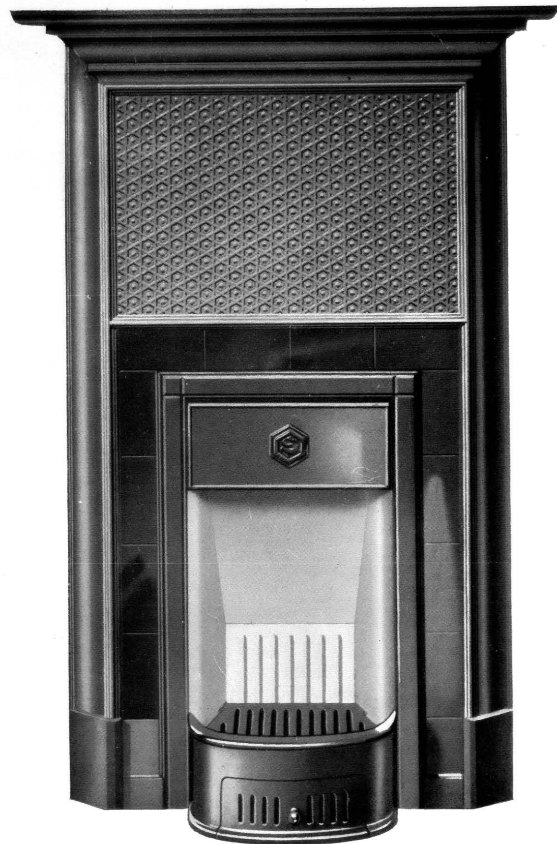
No. 745 TILE MANTEL GRATE, with Double Shelf, Adjustable Cast-iron Canopy, "Vulcan" Fire, with Sliding Draught Regulator, Brick Back in four pieces. Prepared for 3 in. Tiles.
