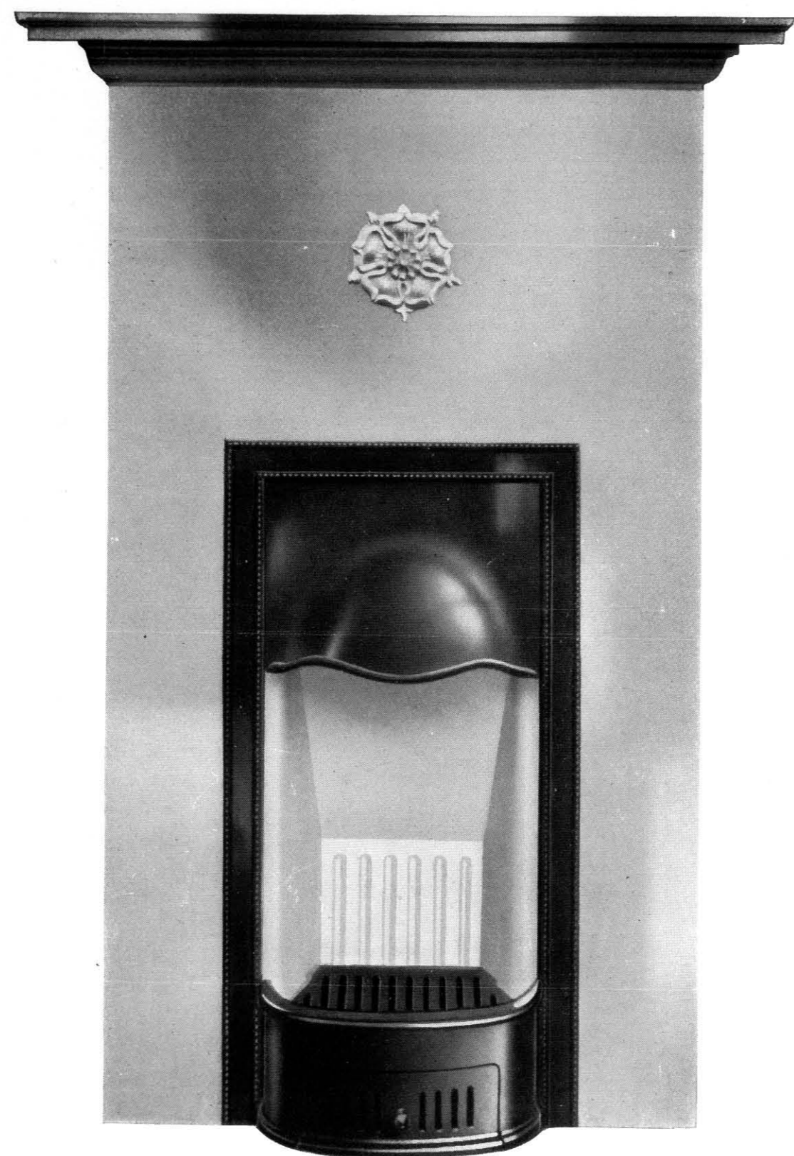
No. 737 MANTEL GRATE, with Single Shelf, Adjustable Cast-iron Canopy, "Vulcan" Fire, with Sliding Draught Regulator and Brick Back in four pieces.
