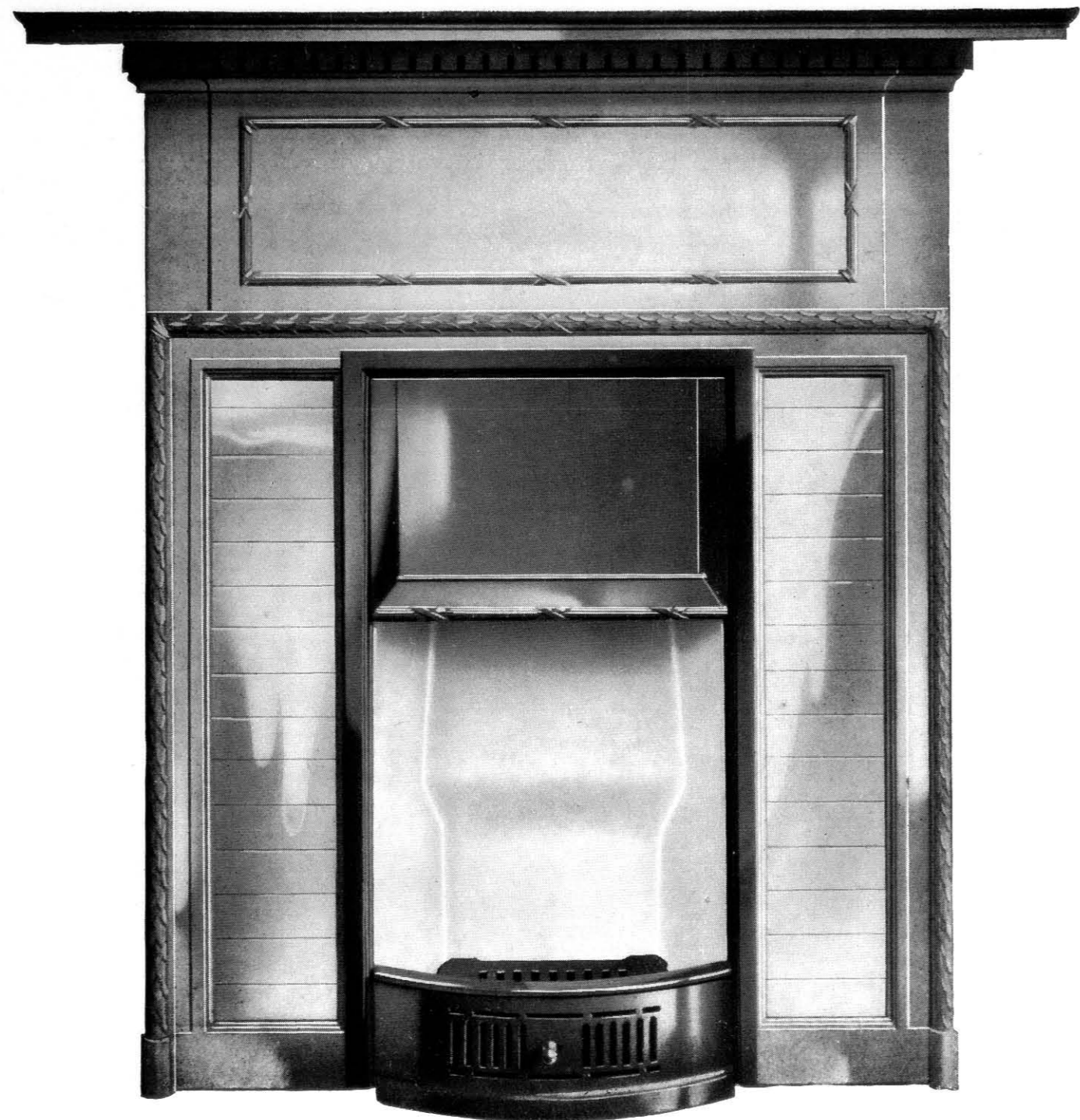
No. 794 TILE MANTEL GRATE, with Single Shelf, Adjustable Cast-iron Canopy, "Douglas" Fire, with Sliding Draught Regulator, W/S Solid Brick Back with Vent Damper. Prepared for Tiles.
