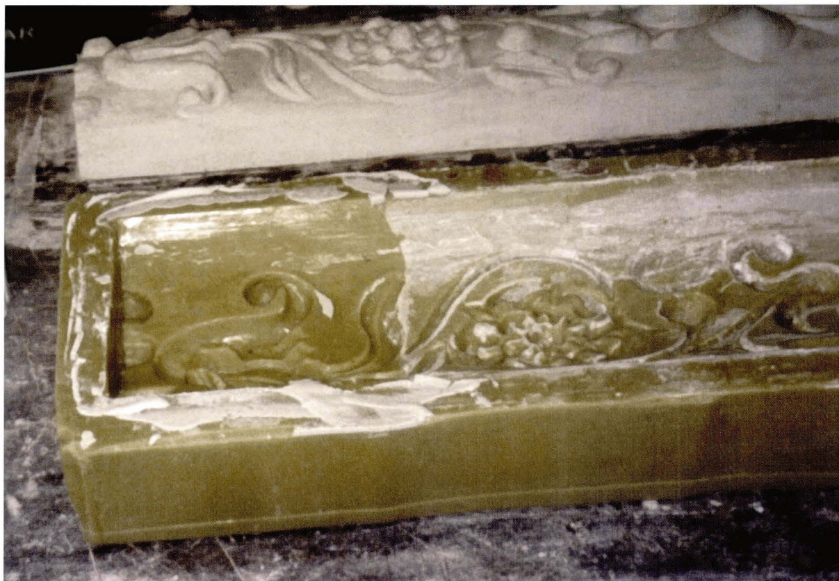
Illus 40. Negative mould and cast. This is a modern flexible mould. Originally wooden moulds would have been used. © Crown copyright Historic Scotland
