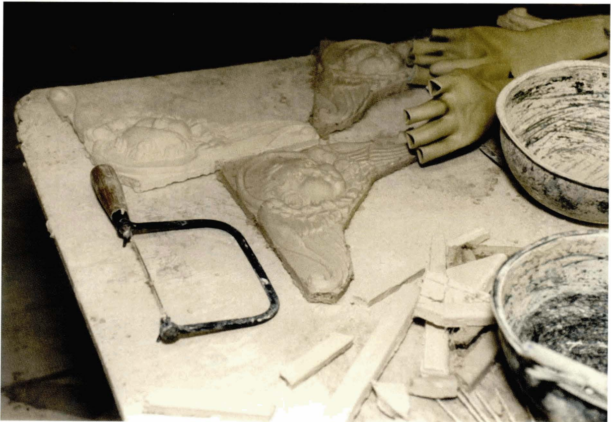
Illus 39. Casting table with casts, rubber gloves, saw and bowls for plaster. © Crown copyright Historic Scotland
