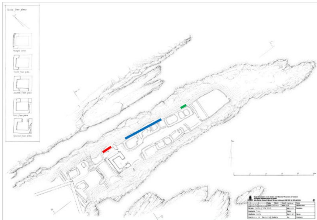
Figure B: Plan of Castle of Old Wick with approximate location and extent of masonry fragments on the north-west cliff face noted, identified in the 2009 survey. Red = masonry fragments 001, 002; blue = masonry fragment 003; green = masonry fragments 004, 005. © Historic Environment Scotland.
