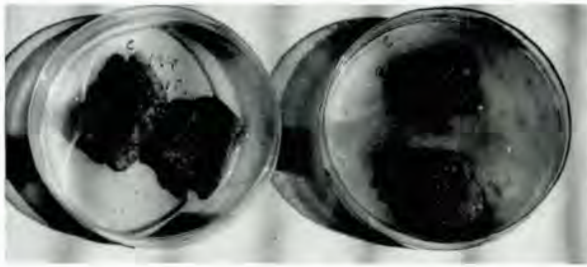
Figure 26a Incubation from light to dark conditions. Control sample on the left. Note the brown slime coating the test sample on the right.
