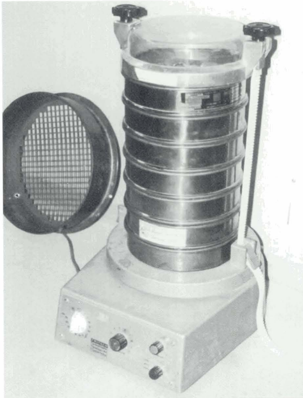
Figure 12 Sieve stack including sieve shaker (sieve shaker courtesy of the British Geological Survey).
