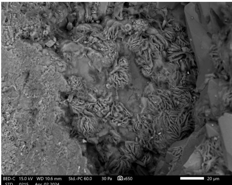
Figure B7. Backscatter electron microscope image of Side A of the fragment (Map area 006). This is a highly compacted area with calcium-rich intergranular material (arrowed) between quartz grains. Grey scale colours correspond to the mean atomic weight of each phase: higher atomic weights (e.g. Ca) being lighter in colour and lower atomic weights (e.g. Si), darker.
