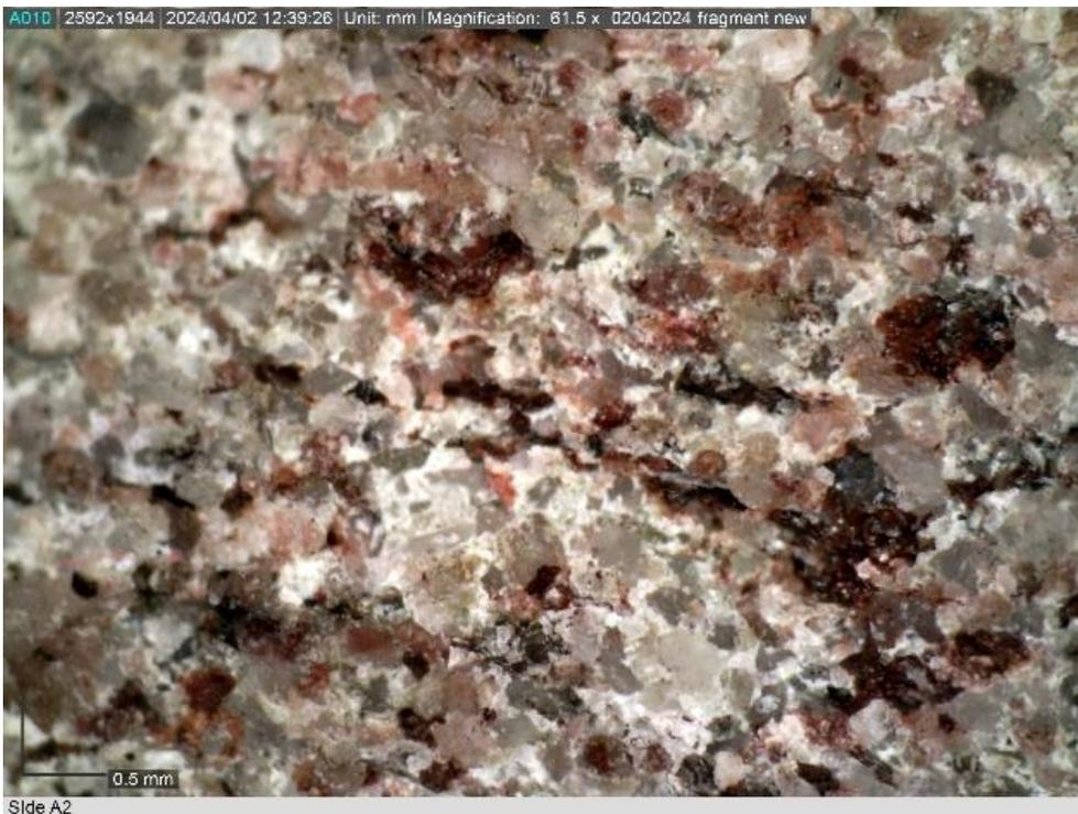
*Figure 4. Stereo microscope image of fragment. The orange-brown patch (lower centre) is an area of probable iron oxide staining on the fragment.*
