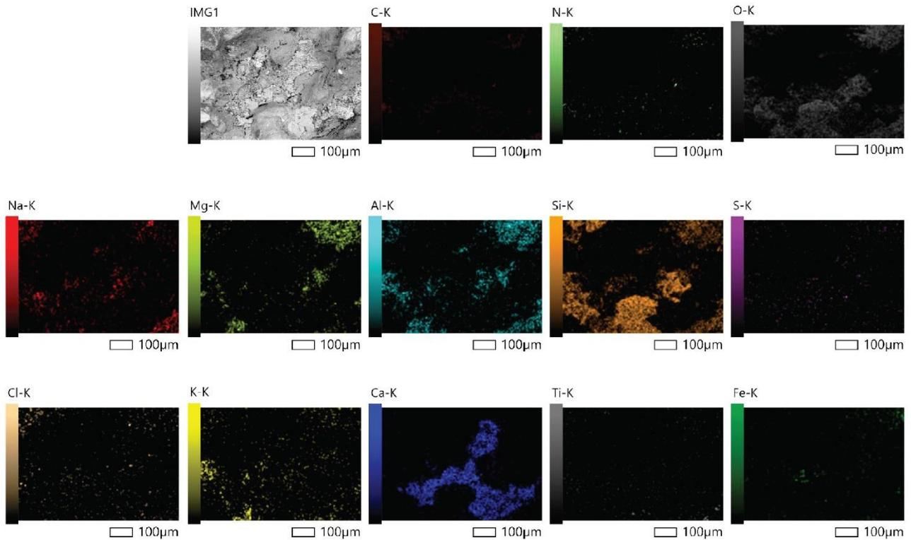
Figure B4. EDS spectrum for Map area 006. Peaks indicate detection of various chemical elements.
