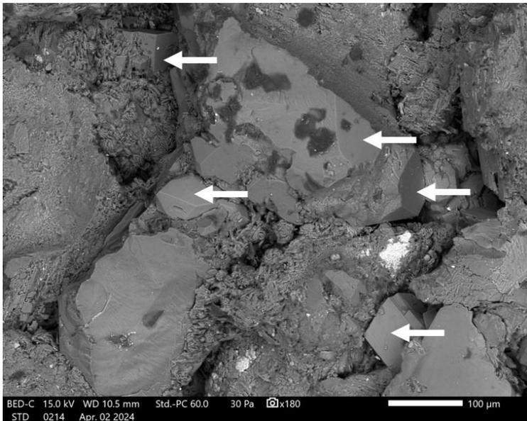
Figure B6. Backscatter electron microscope image of Side A of the fragment. Platy textures consistent with clays are evident throughout the stone, located in regions between detrital grains. Grey scale colours correspond to the mean atomic weight of each phase: higher atomic weights being lighter in colour and lower atomic weights, darker.
