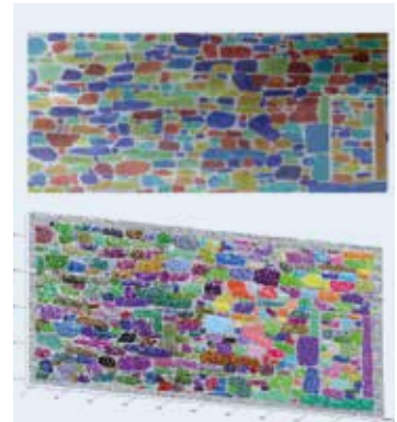
Results of the HWU algorithm, which classifies the 3D data into either stone or mortar joints (courtesy of HWU)
