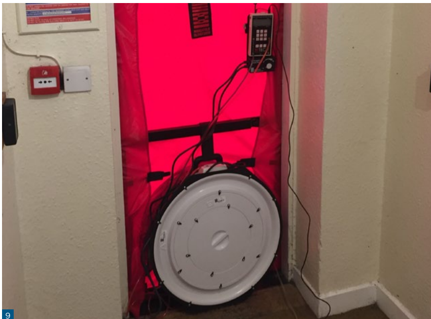
Figure 9: An air pressure test taking place at Holyrood Park Lodge before the interventions.
