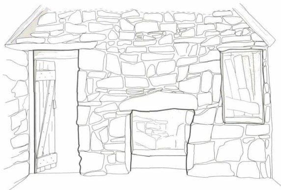
Illus 46 A typical partition wall with door, fireplace and shelves (drawn by Margaret Engl).
