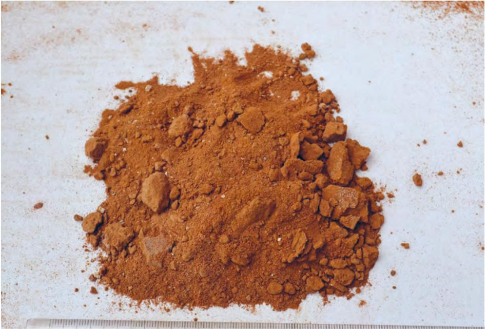
*Fig. 6 Old clay mortar is often soft and can be easily broken down.*
