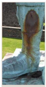
Wrought iron armature captured in bronze during casting, subsequently corroding © D S Mitchell
