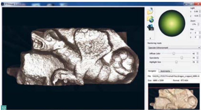
Fig. 32 RTI dataset visualised with specular enhancement shader.
