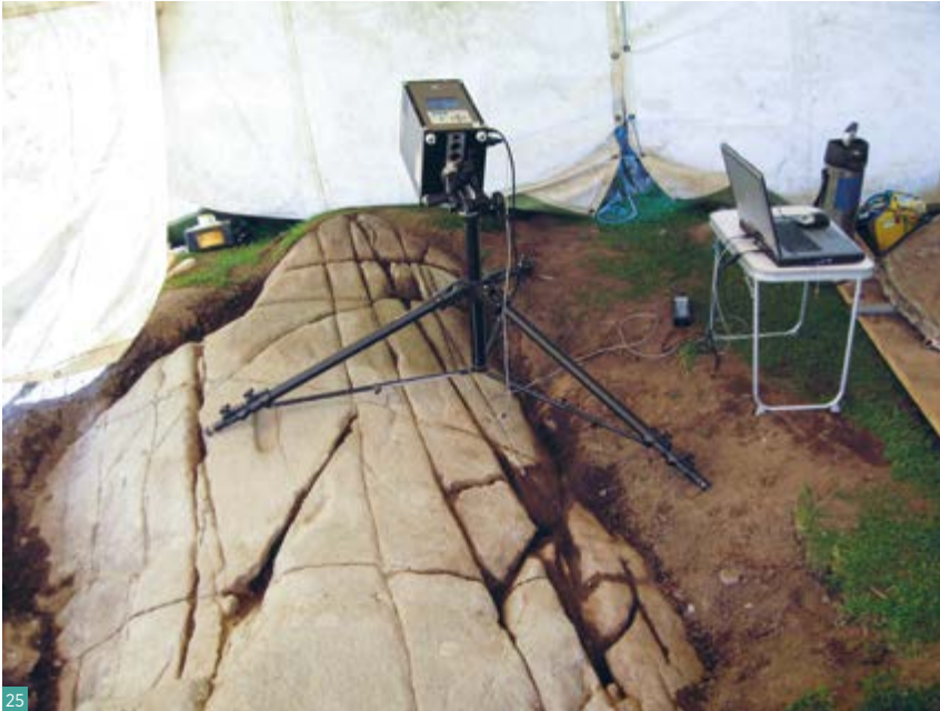
Fig. 25 Konica Minolta VIVID 9i used to scan Dunadd's ogham inscribed stone in Argyll.
