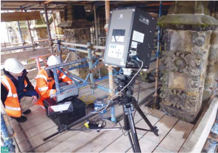
Fig. 54a Laser scanning a Rosslyn Chapel turret with the Konica Minolta VIVID 9i for condition monitoring.
