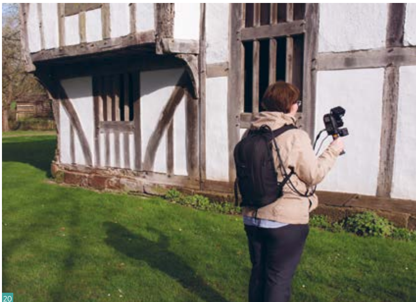
Fig. 20 Undertaking data capture on-site via SLAM with the Zeb-Revo. Image courtesy of Historic England.
