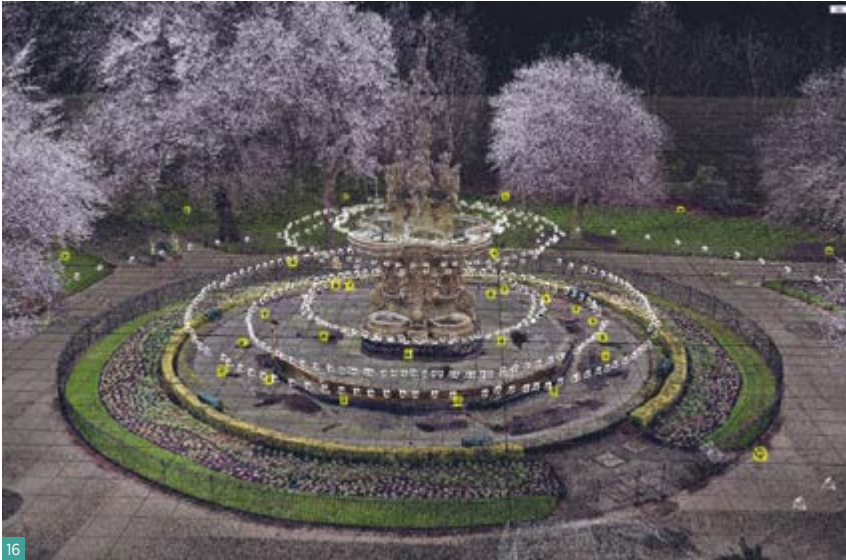
Fig. 16 Preview of alignment between terrestrial laser scanning data and SfM of Ross Fountain, Edinburgh. Scan setups are indicated with yellow-outlined cubes, photographs by white-outlined pyramids showing camera orientation.
