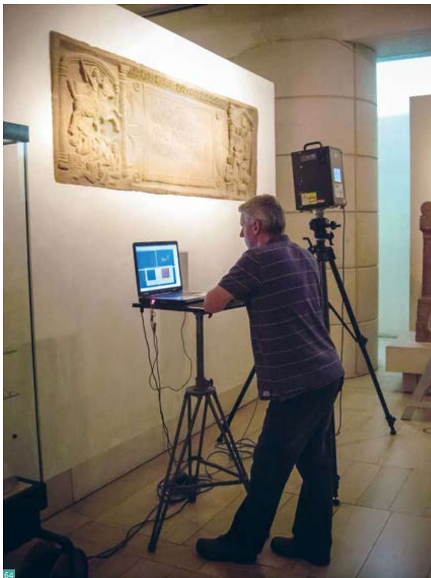
Fig. 64 Capturing the Bridgeness slab with a Konica Minolta VIVID 9i triangulated laser scanner.
