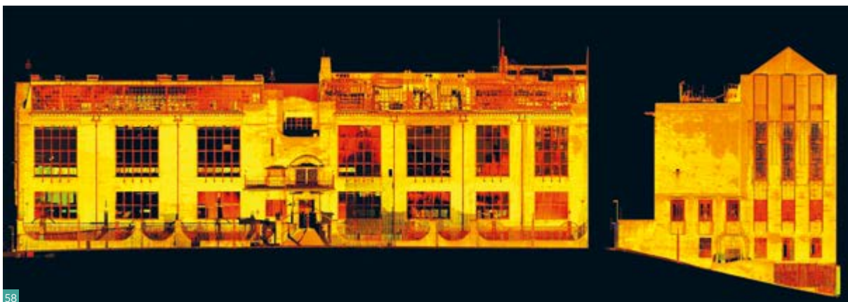
Fig. 58 Laser scan data from the post-fire Glasgow School of Art Mackintosh building exterior.
