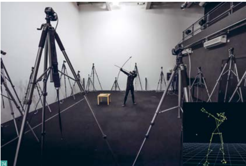
Fig. 74 The motion capture setup used to record and map the animated movement of characters in the game world.
