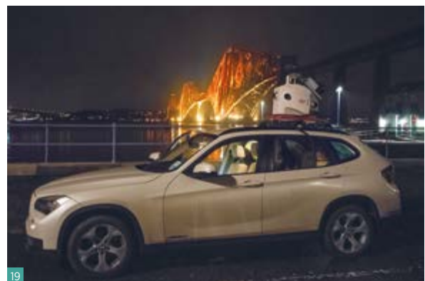
Fig. 19 Leica Geosystems Pegasus car mounted laser profiler.
