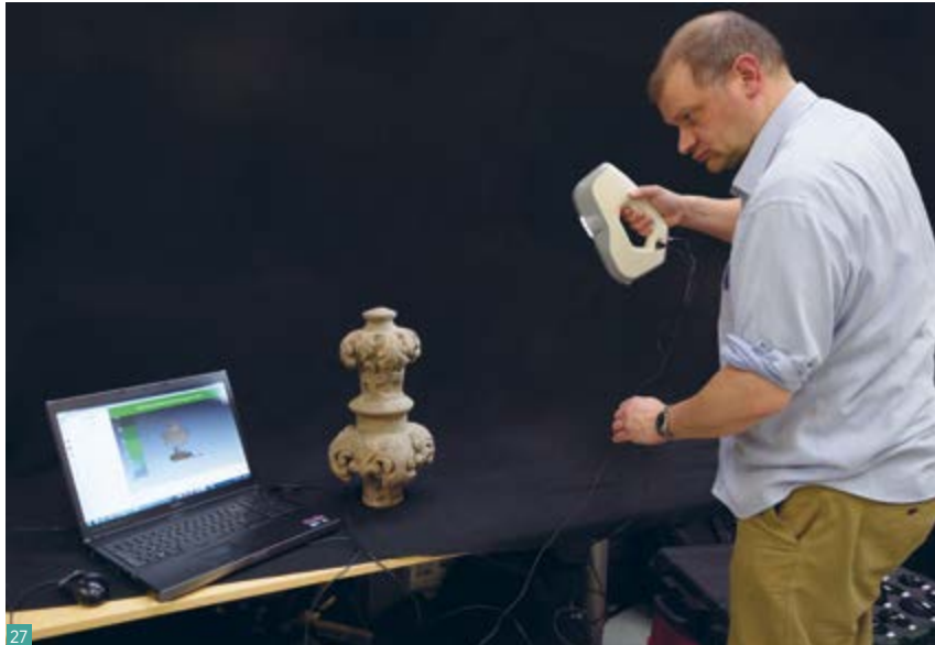
Fig. 27 Structured light scanning using an Artec EVA.
