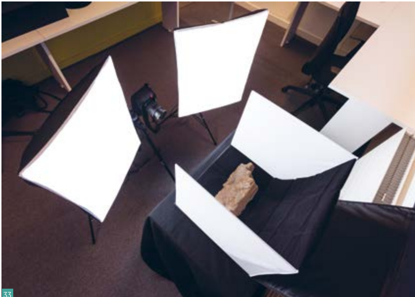
Fig. 33 Photograph of an example photogrammetry setup. The softbox can be used to diffuse and block uncontrolled light.
