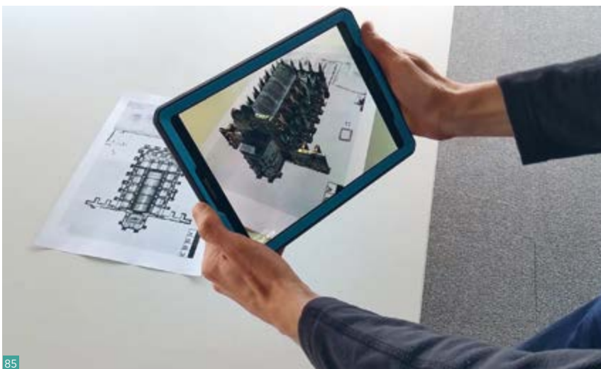
Fig. 85 Augmented reality application overlaying a 3D model of Rosslyn Chapel on top of a tracked 2D target.
