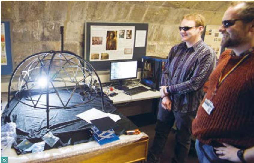
Fig. 28 Framework for geodesic RTI dome using 65 LED lights. Image courtesy of Kirk Martinez, University of Southampton.
