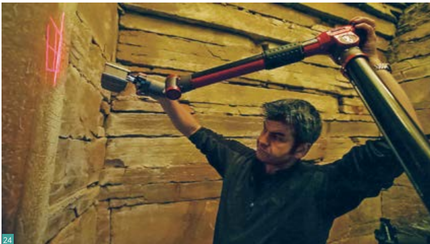
Fig. 24 Arm-mounted triangulated laser scanner being used to capture runic inscriptions at Maeshowe Neolithic chambered tomb in Orkney.
