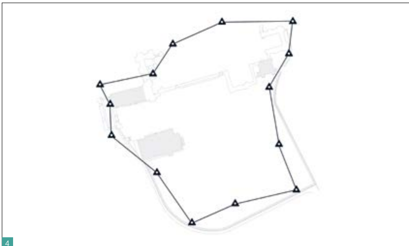
Fig. 4 Illustrative diagram of a closed-loop traverse comprised of 14 setups. Setup positions are marked with triangular icons.
