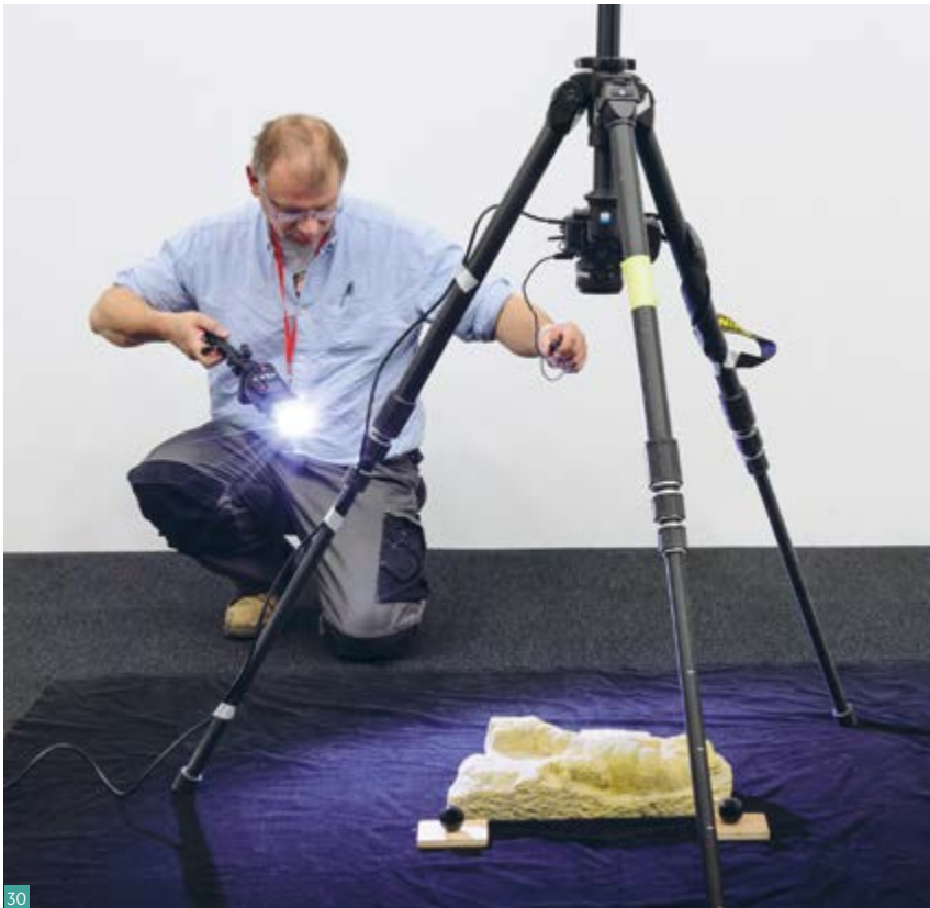
Fig. 30 RTI capture of a carved stone object.
