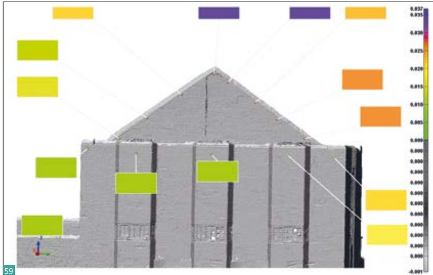
Fig. 59 Deviation map from the Glasgow School of Art's Mackintosh building with point measurements taken from specific stones. Differences calculated between two scans, pre-fire (2008) and post-fire (2014). Green and yellow signify movement of <20mm on the x-axis, purple and orange signify movement of >20mm on the x-axis.
