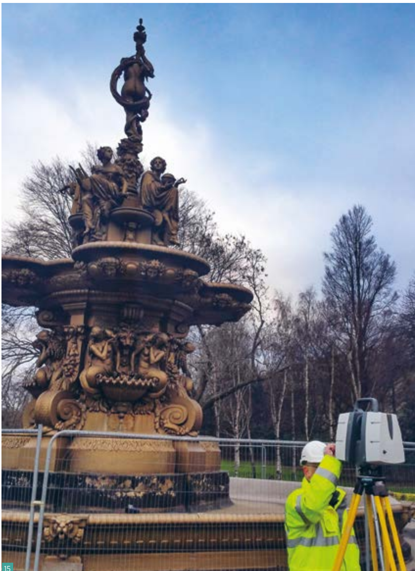
Fig. 15 Terrestrial laser scanning at Ross Fountain, Edinburgh. This data was supplemented with additional data captured via SfM photogrammetry.
