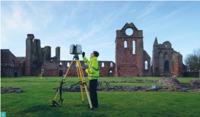
Fig. 6 Terrestrial laser scanning at Arbroath Abbey.
