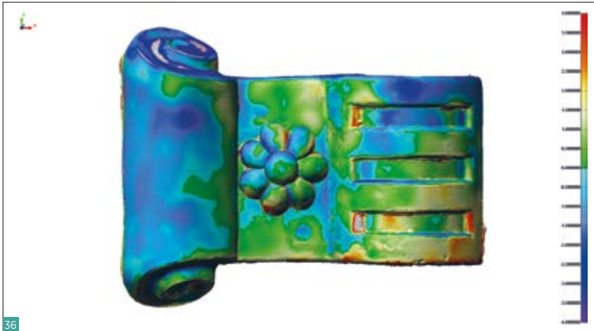
Fig. 36 Deviation map showing extent of difference between laser scan data mesh and modelled component. Red, yellow and green areas correspond to accretion or expansion, blue and purple denote loss or shrinkage.
