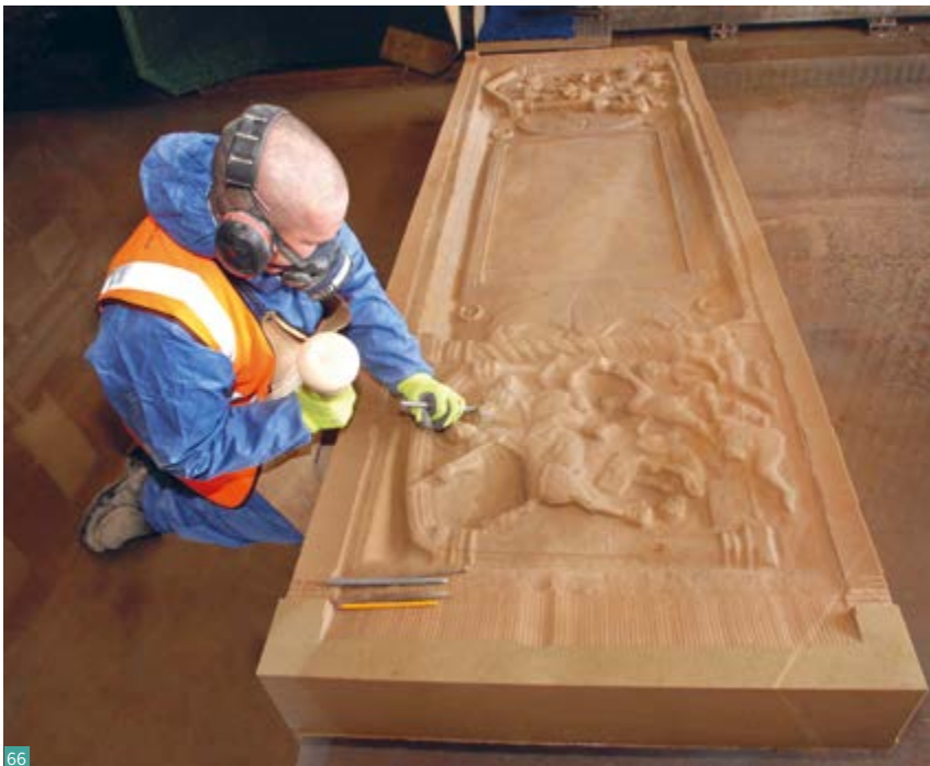
Fig. 66 The CNC milled Bridgeness slab stone being finished by hand. Image courtesy of Falkirk Council.
