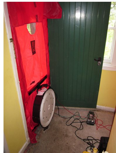
Right: Blower door in situ at Scotstarvit Tower Cottage
