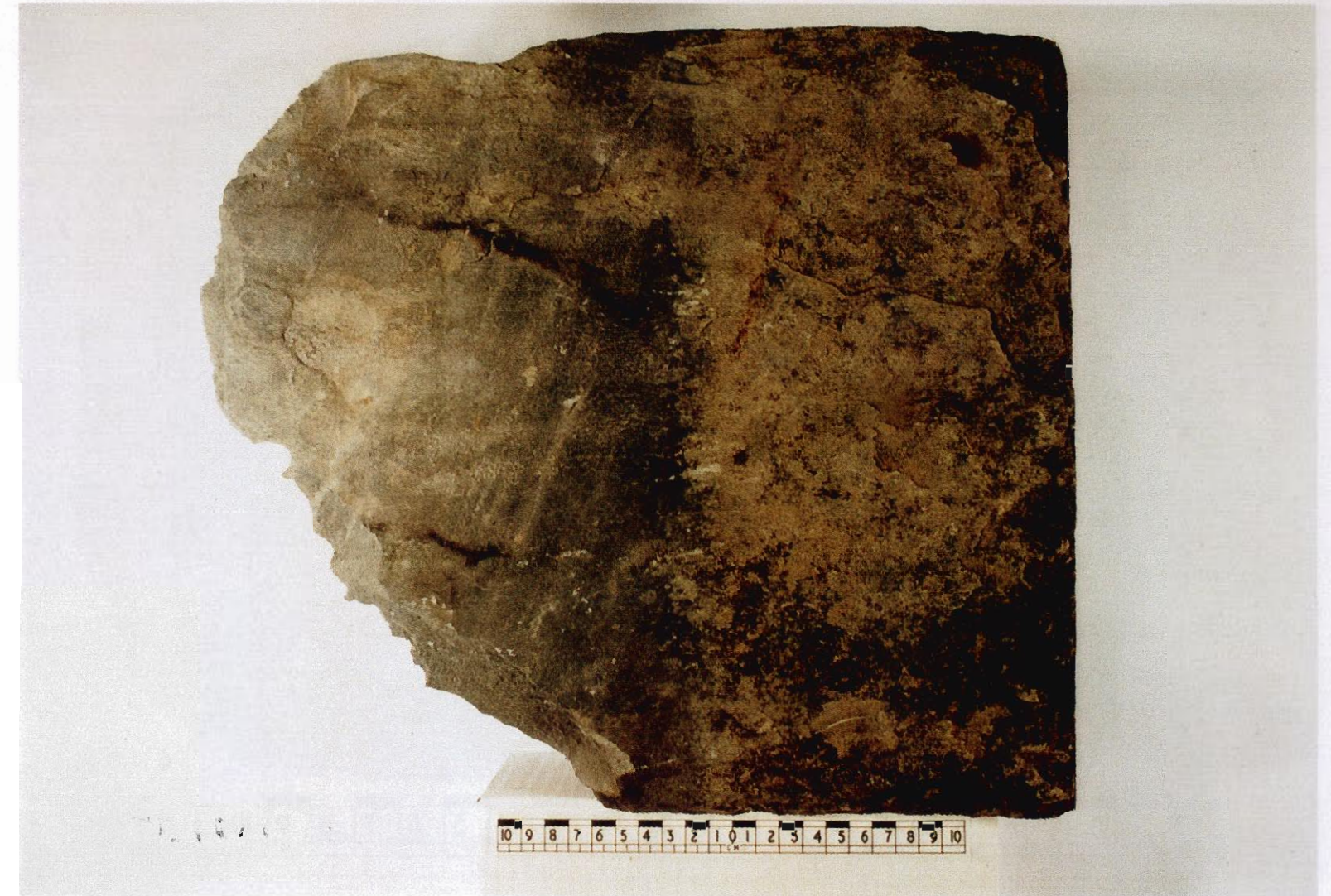
Plate 65 Dunkeld slate from a used slate dealer estimated at over 100 years old
