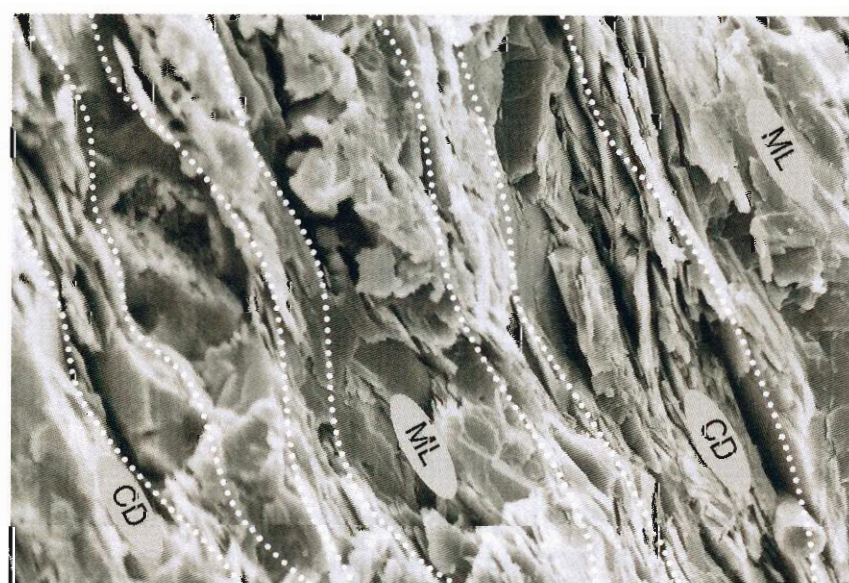
e) FOUDLAND QUARRIES MF-2 Fairly widely spaced, slightly anastomosing around microlithon with some development of fabric estimated thickness 6.0mm.
