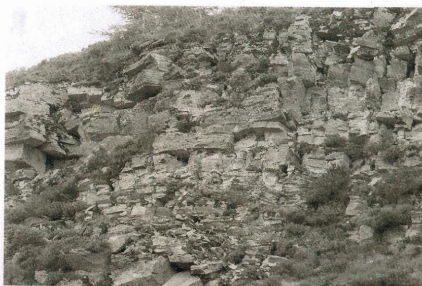
Plate 49 Kirkney Quarry. The overhanging face has collapsed with time, along the pillaring line (NJ503317 to 510320)
