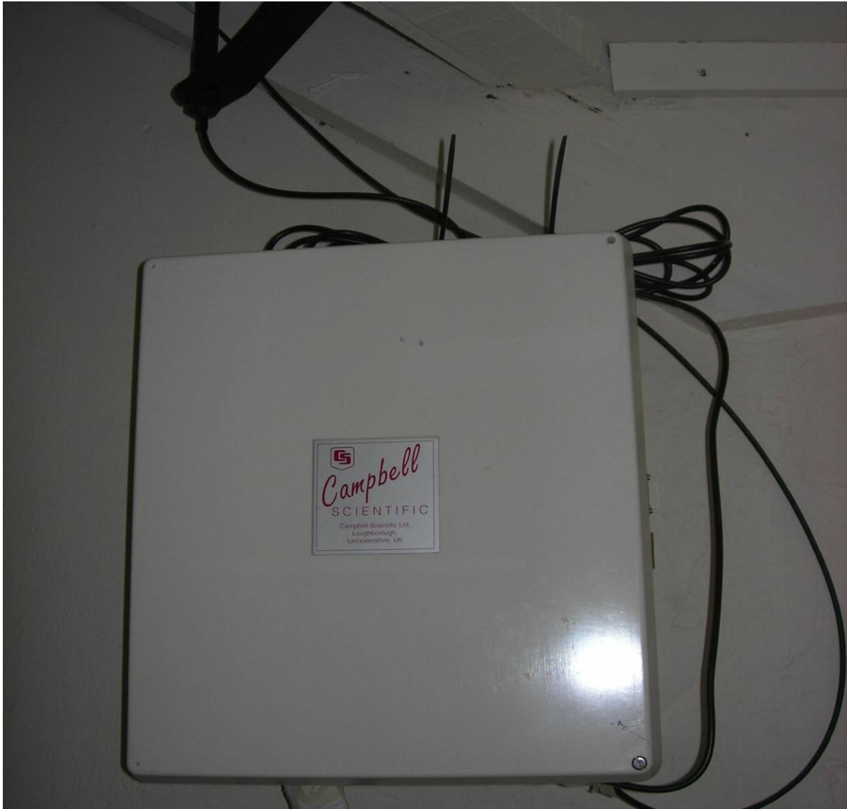
Fig. 18. Remote logging equipment for long term monitoring of hygrothermal performance
