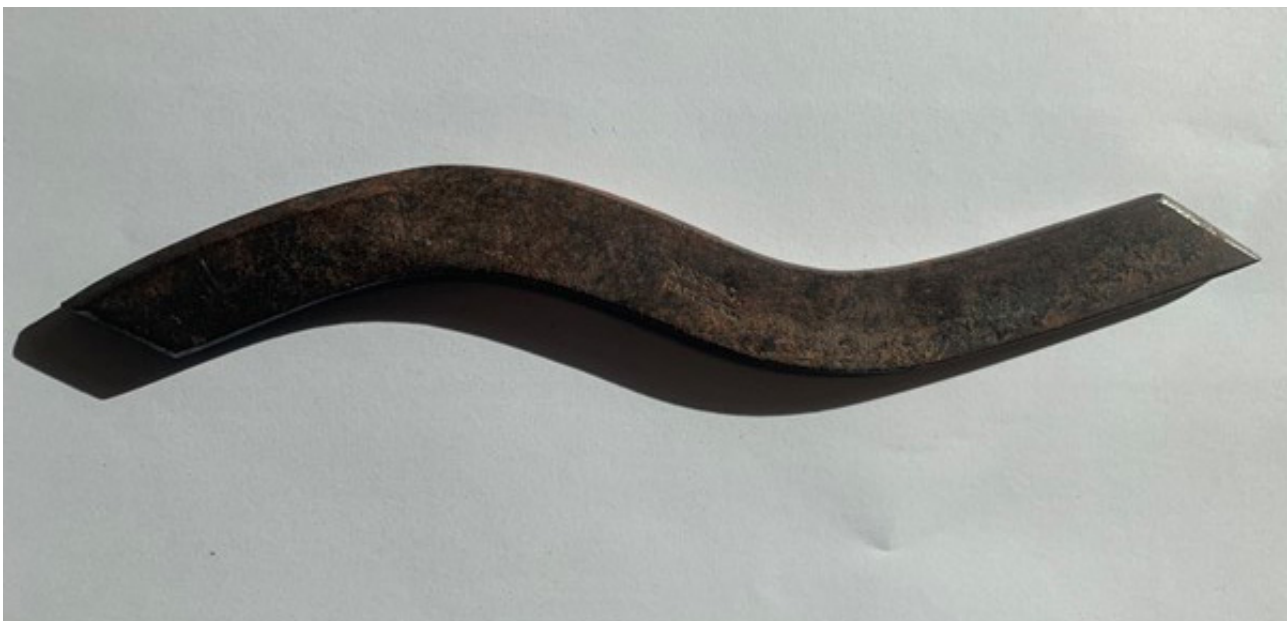
Figure 1 - A ruling out tool from the 19th century. The manufacturer's mark, indicating production at scale, is just visible in the centre.
