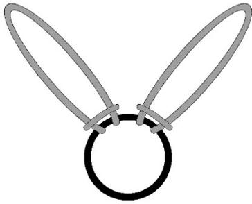
Figure 9 The use of rope slings to lift and move the Stone. © Peter Hill.
