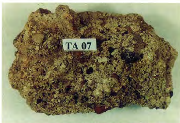
Figure 5.5: Historic mortar sample from Tantallon Castle, East Lothian. The paper label attached to the sample is around 3 cm across. The general texture of this internal fracture surface of an historic mortar (early 16th Century) can be seen clearly. Poorly sorted aggregate contains rounded dark basaltic rock fragments and red coloured intermediate to siliceous extrusive igneous rock fragments. There are also some more angular fragments of charcoal in this specimen.
