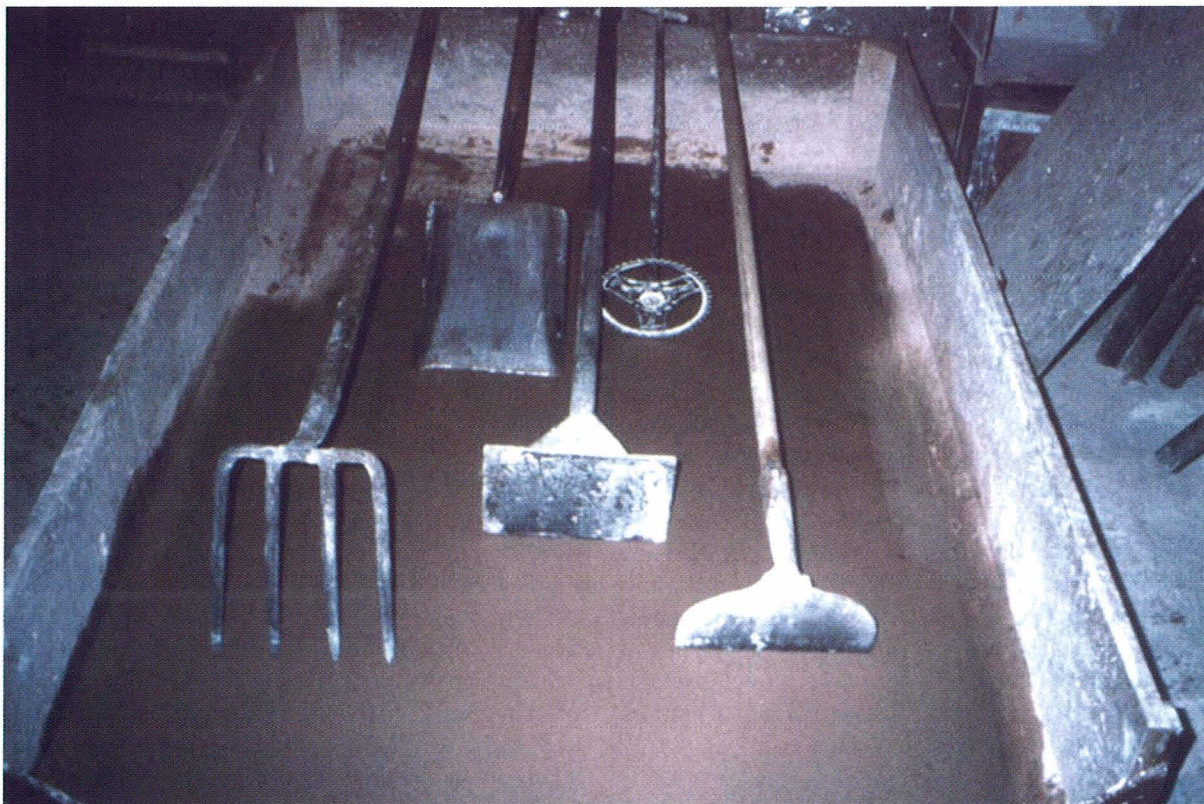
13. Traditional mortar trough and mortar making tools.
