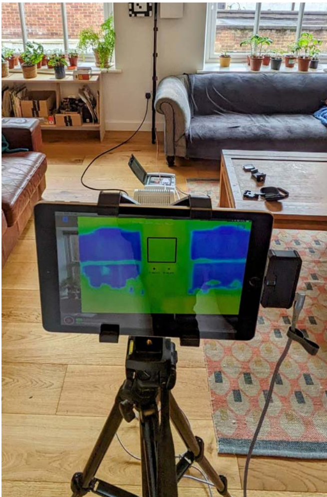
Left: In-situ U-value testing.
