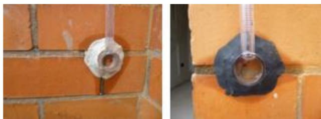
Figure 105 Spread of water along an absorbent joint
