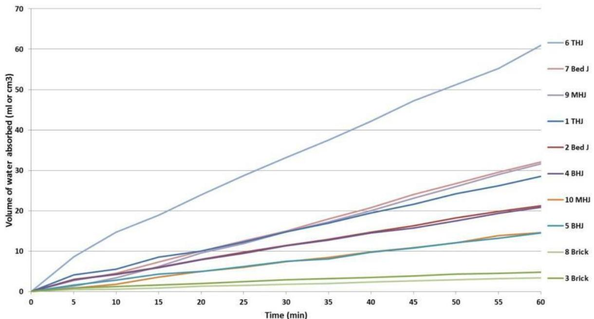
Figure 102 Absorption progression for each location tested on an exposed brick wall of a house in Dublin: The lower two graphs (green) represent measurements made directly on brick surfaces, the others were taken from mortar joints.
