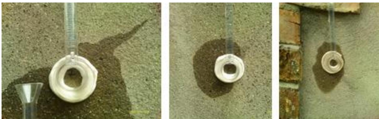
Figure 107 The water absorption pattern in render is totally different.
