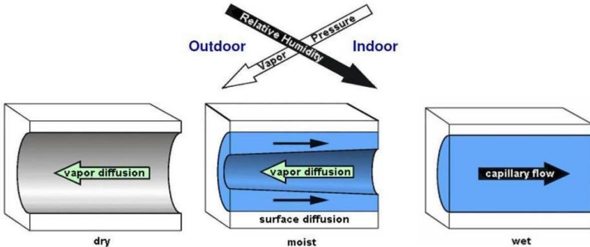
Figure 26 The three different water transport mechanisms possible in a porous, hygroscopic material: vapour diffusion, surface diffusion (of liquid water) and capillary action (also of liquid water). (Fraunhofer IBP / Image © Fraunhofer-Gesellschaft)
