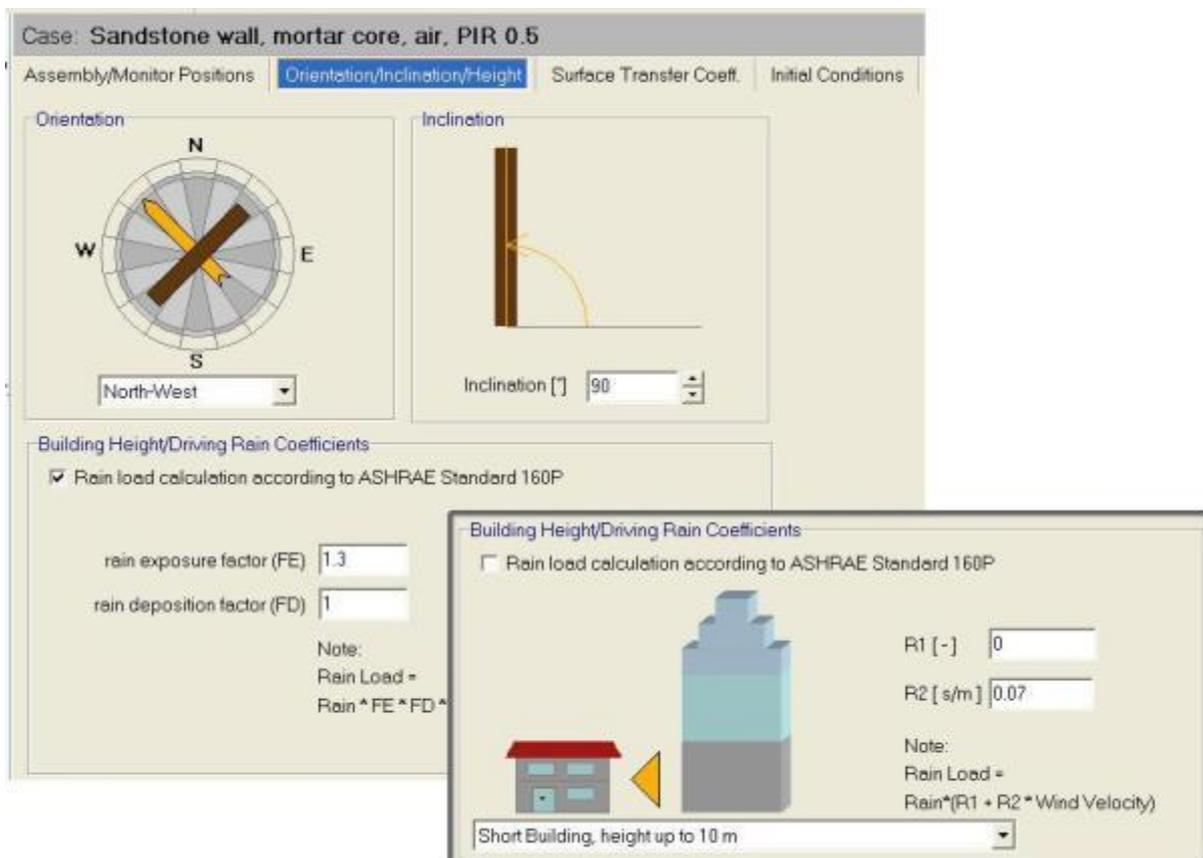
Figure 64 WUFI Pro screenshot showing selections possible to localise selected climate data for a specific building element, including orientation, inclination, height above ground and wind-driven rain coefficient
