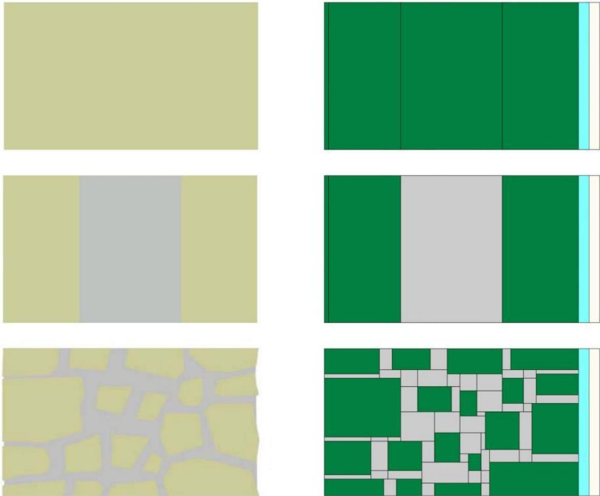
Figure 82 Three conceptual geometrical models of the existing wall and their translation into WUFI simulation models, with increasing levels of accuracy starting at the top (compare to Figure 69)
