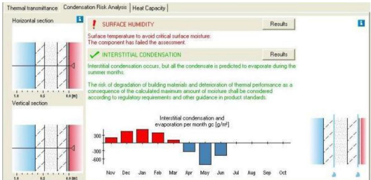
Figure 74 BuildDesk U screenshot showing the results from the Glaser method assessment of the base, for a *high occupancy* setting.
