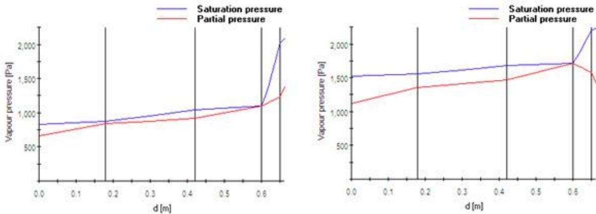
Figure 45 Example of Glaser method diagrams showing partial and saturation pressure profiles across a cross section of building fabric: the left diagram shows profiles for February, indicating interstitial condensation at the location where profile lines meet. The June profiles (right) indicate evaporation.
