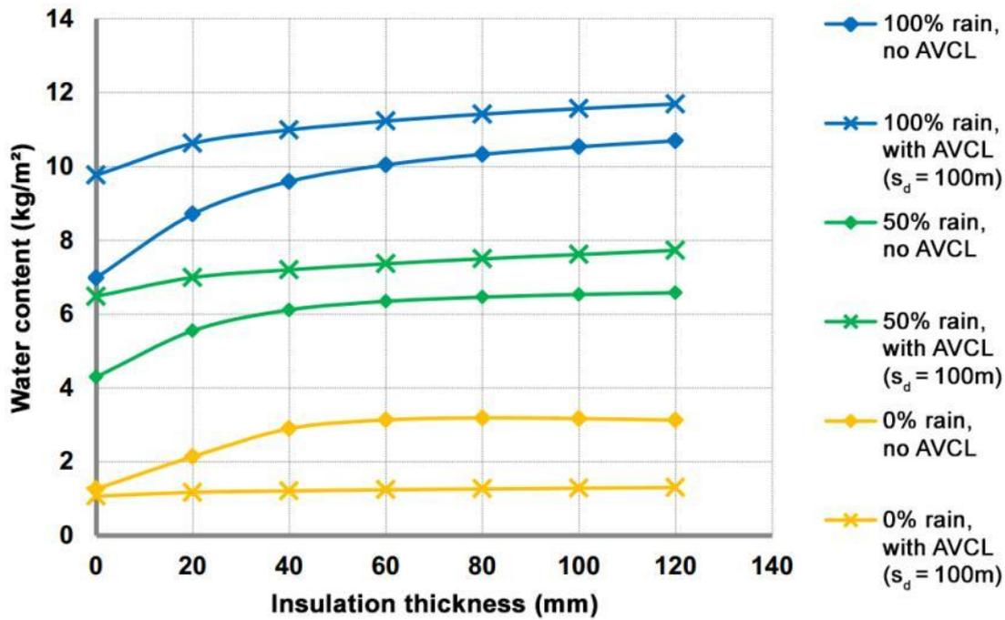
Figure 97 Average total water content (from hygrothermal simulation) of an existing exposed brick solid wall internally insulated with mineral wool insulation, as a function of insulation thickness (x axis), driving rain absorption (colour code) and presence or absence of an AVCL (point shape). (Image © Worch)
