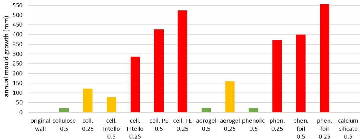
Figure 91 Predicted annual mould growth, using biohygrothermal modelling with WUFI-Bio for the Stone A solid wall substrate
