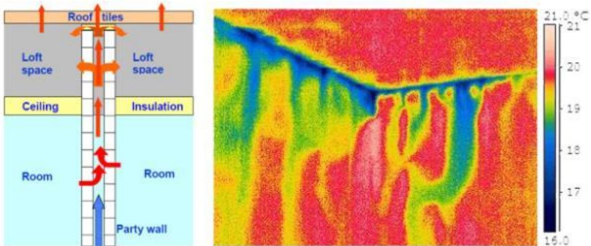
Figure 35 On-site investigations at a housing development in Stamford Brook, London, found that convective heat loss occurred, on one hand, due to heat transfer from rooms either side of a party wall, with a convection current in the wall's cavity causing the air to rise to the colder, uninsulated attic space (left), and, on the other hand, due to air movement behind mechanically fixed plaster-board dry-linings. (Wingfield et al., 2011 / Image © DCLG)
