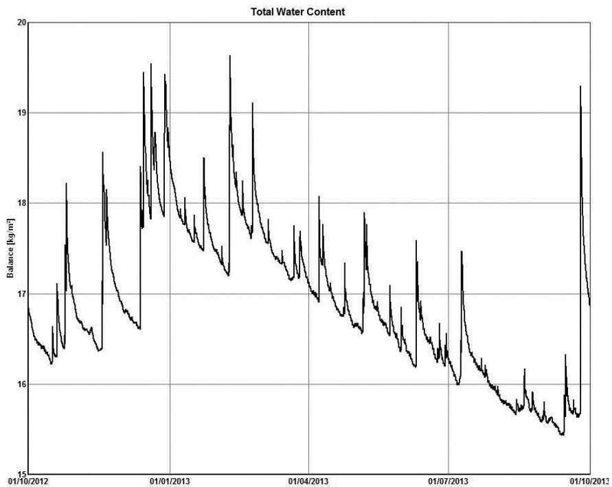
Figure 78 Fluctuation of total water content of the base wall, as simulated with WUFI for the period of one year.
