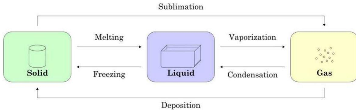
Figure 13 Physical states of matter and terms related to the phase transitions (compare to Figure 15). (ElfQrin, 2011 / Image © ElfQrin CC BY-SA 4.0)
