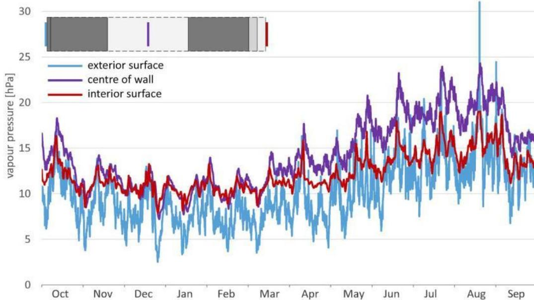
Figure 81 Vapour pressures at the exterior and interior surfaces of the wall and at the centre of its mortar core layer
