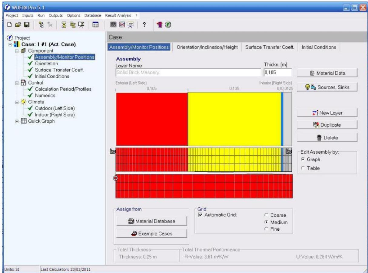
Figure 48 Screenshot of WUFI Pro 5.1: the software uses variable-sized, computational grid elements to assess the cross section of a construction. Denser grid elements are used at the inside and outside surface of the construction and at the material interfaces.
