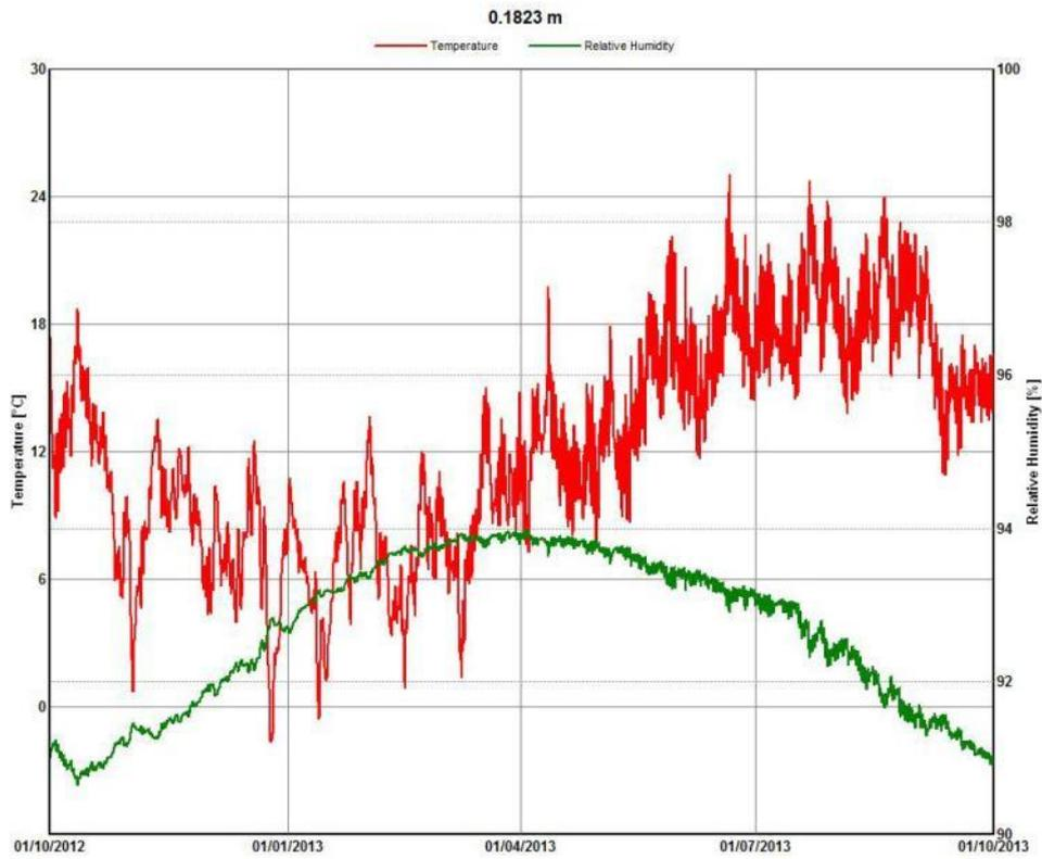
Figure 77 Temperature and relative humidity, as simulated with WUFI for one year, at the interface between the external stone and mortar core layers.
