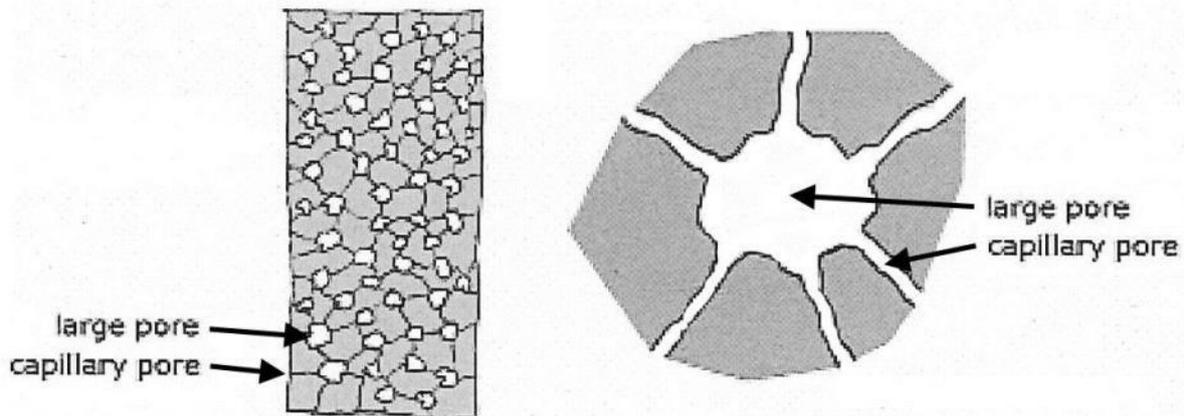
Figure 9 Sketch illustrations of a material's pore structure: the right illustration is a magnification of the left, showing a large pore with connected capillary pores. (Torraca, 2009, p.82, fig. 3.19 / Image © The J. Paul Getty Trust)
