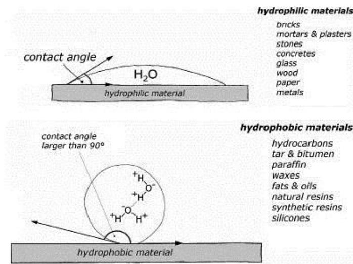
Figure 16 Graphic illustrations of hydrophilic and hydrophobic material surfaces (Torraca, 2009, p. 36, fig. 1.74 and 1.75 / Image © The J. Paul Getty Trust)
