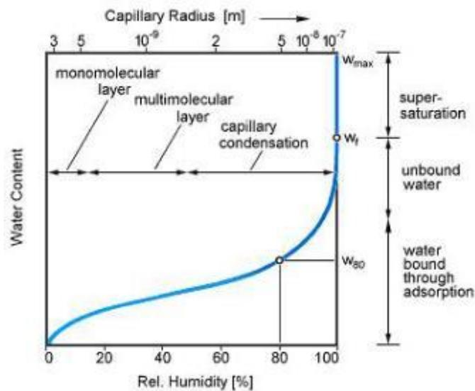
Figure 27 Moisture storage function curve of a material (Fraunhofer IBP / Image © Fraunhofer-Gesellschaft)
