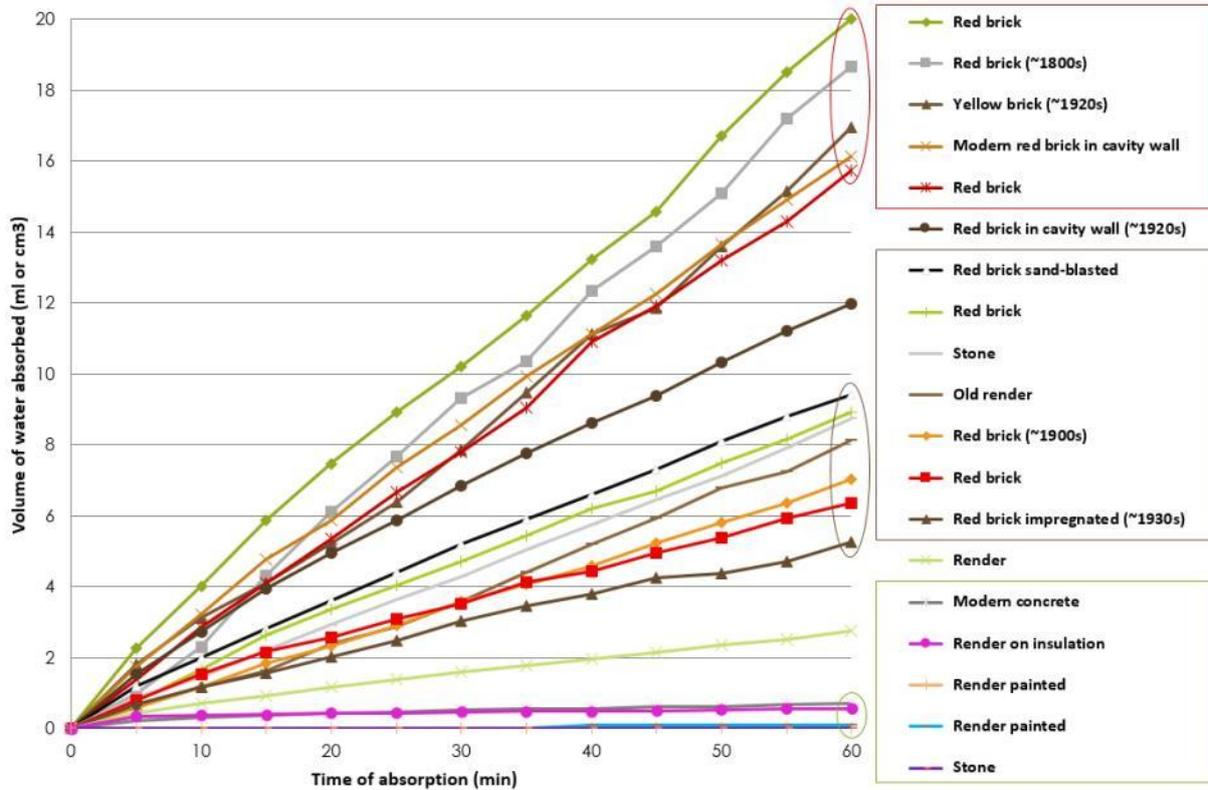
Figure 103 Absorption of a range of different buildings tested in Dublin: the mean progression is shown for each wall
