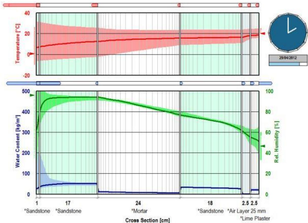
Figure 79 WUFI screenshot showing relative humidity, temperature and water content profiles of the base wall, taken as a snapshot at a single one-hour time-step in April.
