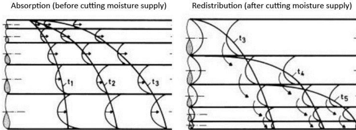
Figure 25 Capillary transport phenomena represented by a model of interconnected cylindrical capillaries of various diameters (Fraunhofer IBP / Image © Fraunhofer-Gesellschaft)
