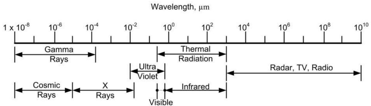
Figure 11 The electromagnetic spectrum is a logarithmical scale
