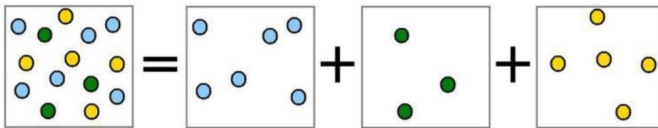
Figure 17 Diagram illustrating the relationship of overall and partial gas pressures: the total gas pressure is the sum of the partial pressures of each particular gas.
