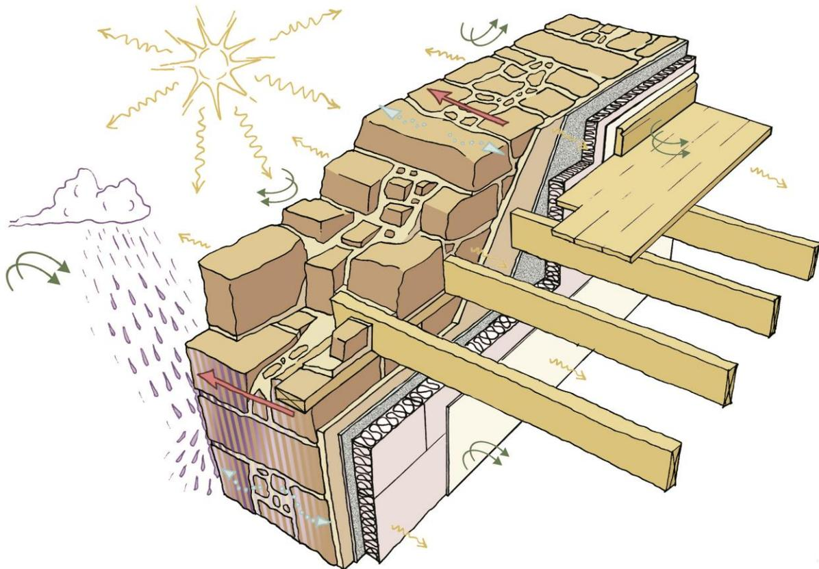
Figure 95 A graphic representation of a *moisture managing* internal wall insulation system featuring a fully-bonded, hygroscopic and capillary active insulation assembly
