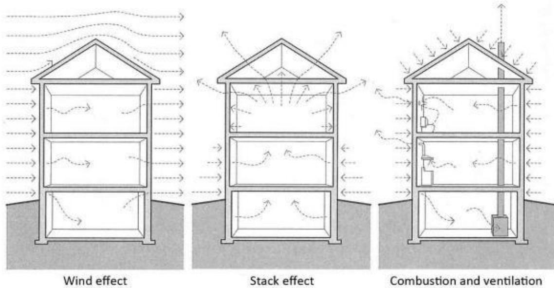
Figure 3 Natural and man-made forces driving air flow through building envelopes. (Straube and Burnett, 2055, p272, fig. 7.2 / Image © Building Science Press)
