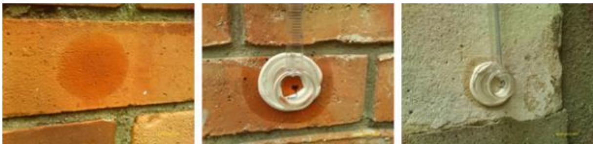
Figure 104 Circular wetting patterns for the homogeneous surface
