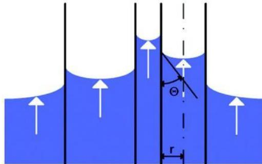
Figure 24 Capillary ascension in ideal material pores due to capillary pressure (Fraunhofer IBP / Image © Fraunhofer-Gesellschaft)
