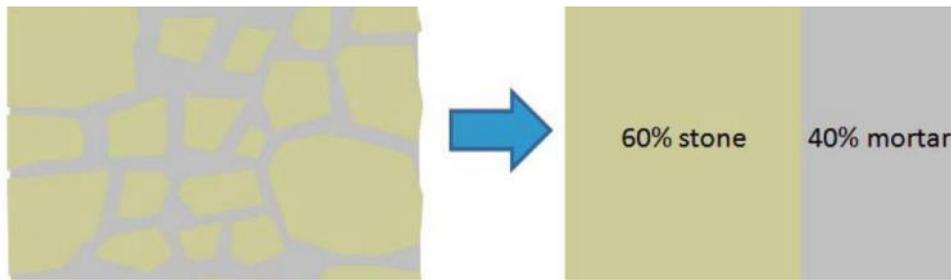
Figure 69 Schematic illustration of a cross section of a solid stone wall (left) and the simplified geometrical model (right) used in Baker (2011) for U-value calculation.
