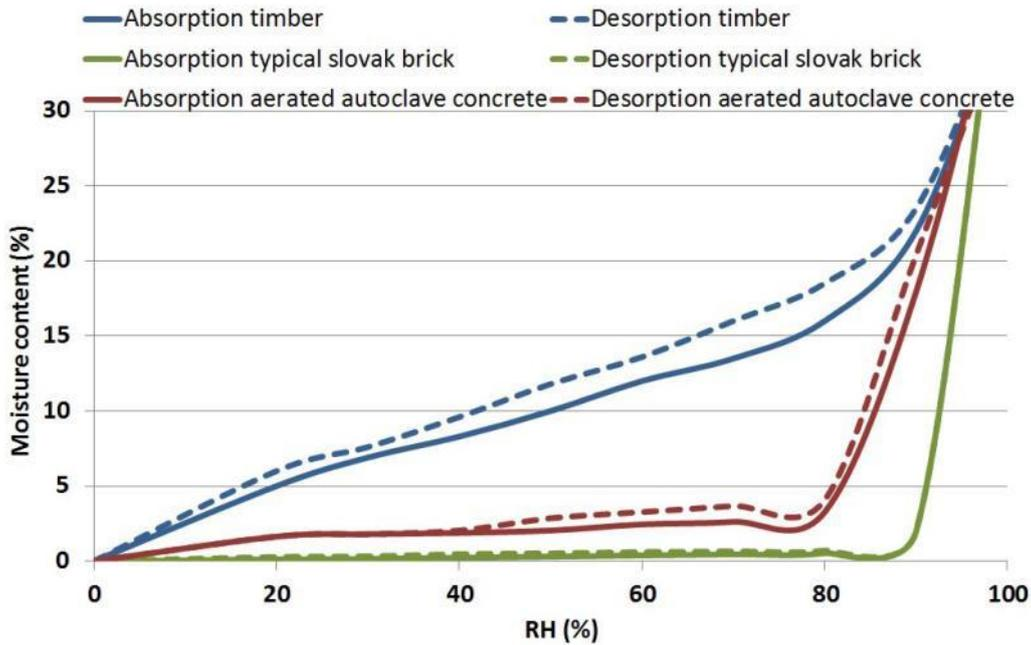
Figure 28 Graphs showing the hysteresis of timber (generalised), of a type of brick and of an aerated autoclave block
