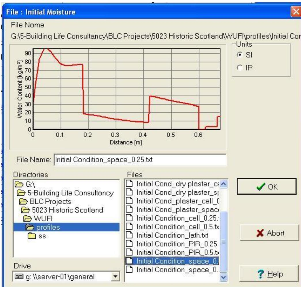
Figure 109 Screen shot of WUFI Pro showing a profile prepared for a simulation start: The graph right of the 0.6 m mark represents the moisture content of the retrofits.
