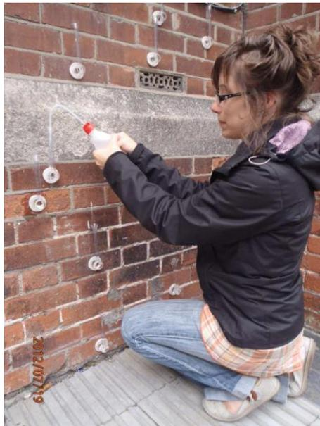
Figure 99 Array of Karsten tubes being filled
