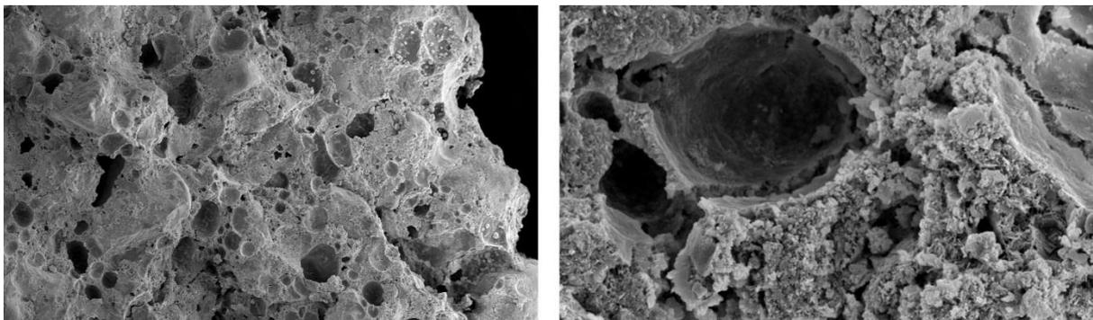
Figure 8 Scanning electron microscope photograph of mortar with 50 x magnification (left) and 2000 x magnification (right)
