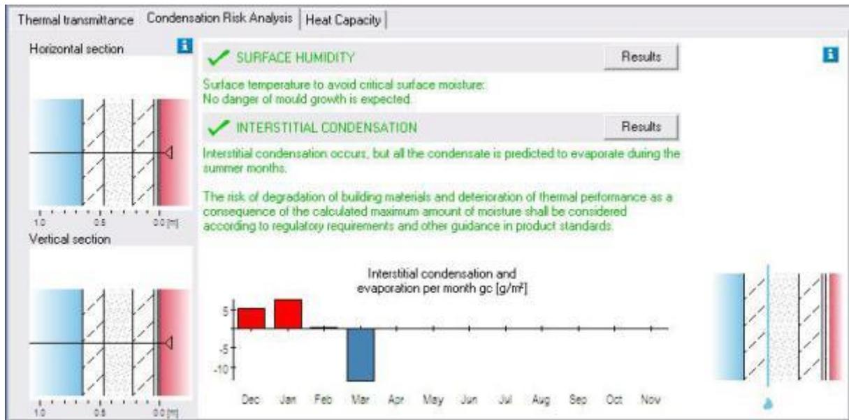
Figure 73 BuildDesk U screenshot showing the results from the Glaser method assessment of the base wall, for a *low occupancy* setting.
