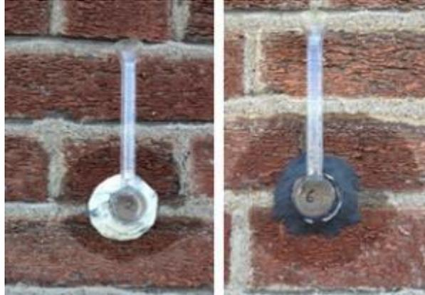
Figure 106 Specific wetting patterns on joint-brick interfaces can appear, as for the Dolphin House's brick wall
