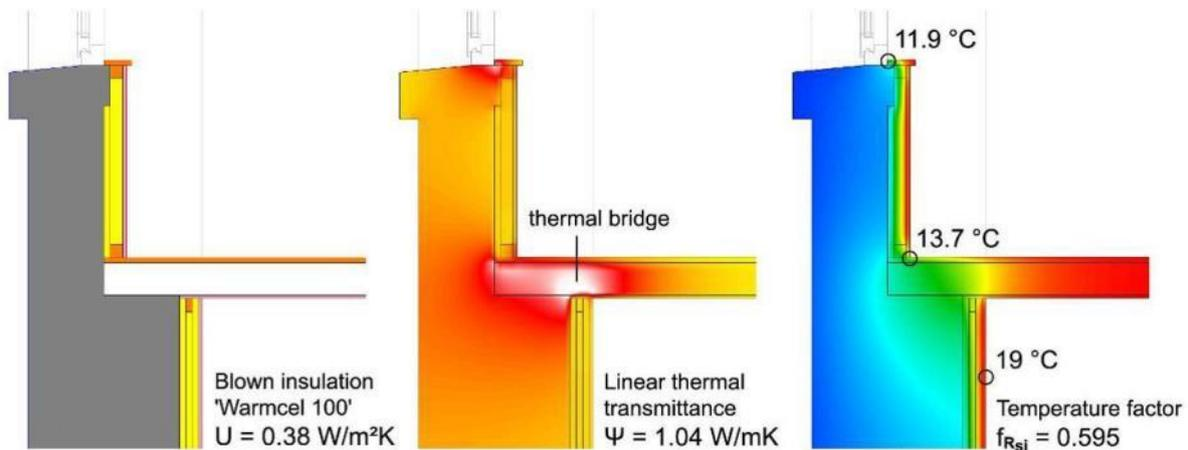
Figure 93 Cross section of a wall with a window breast, which, in comparison to Figure 92, is now retrofitted with internal wall insulation: the location of the most significant thermal bridge is now the floor-wall junction; the cill-window junction remains a thermal bridge also, albeit of lesser significance. Although the surface temperatures have significantly increased, the temperature factor is only marginally higher than in the uninsulated scenario.
