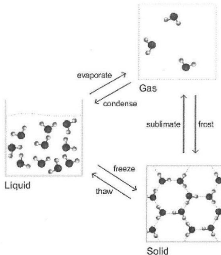
Figure 15 Diagram showing the different physical states of water and the phase transitions processes (compare to Figure 13). (Straube, 2006a, p. 2, fig. 1 / Image © Building Science Press)
