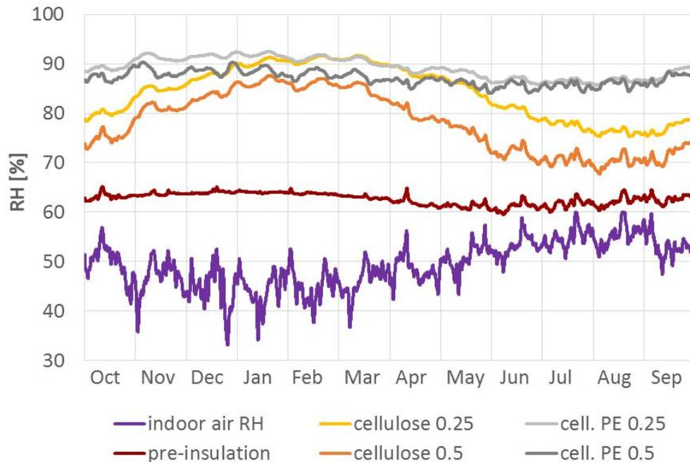
Figure 89 Relative humidity of indoor air and at the insulation-masonry interface prior to retrofit and with four different cellulose fibre retrofit options installed, for the seventh simulation year
