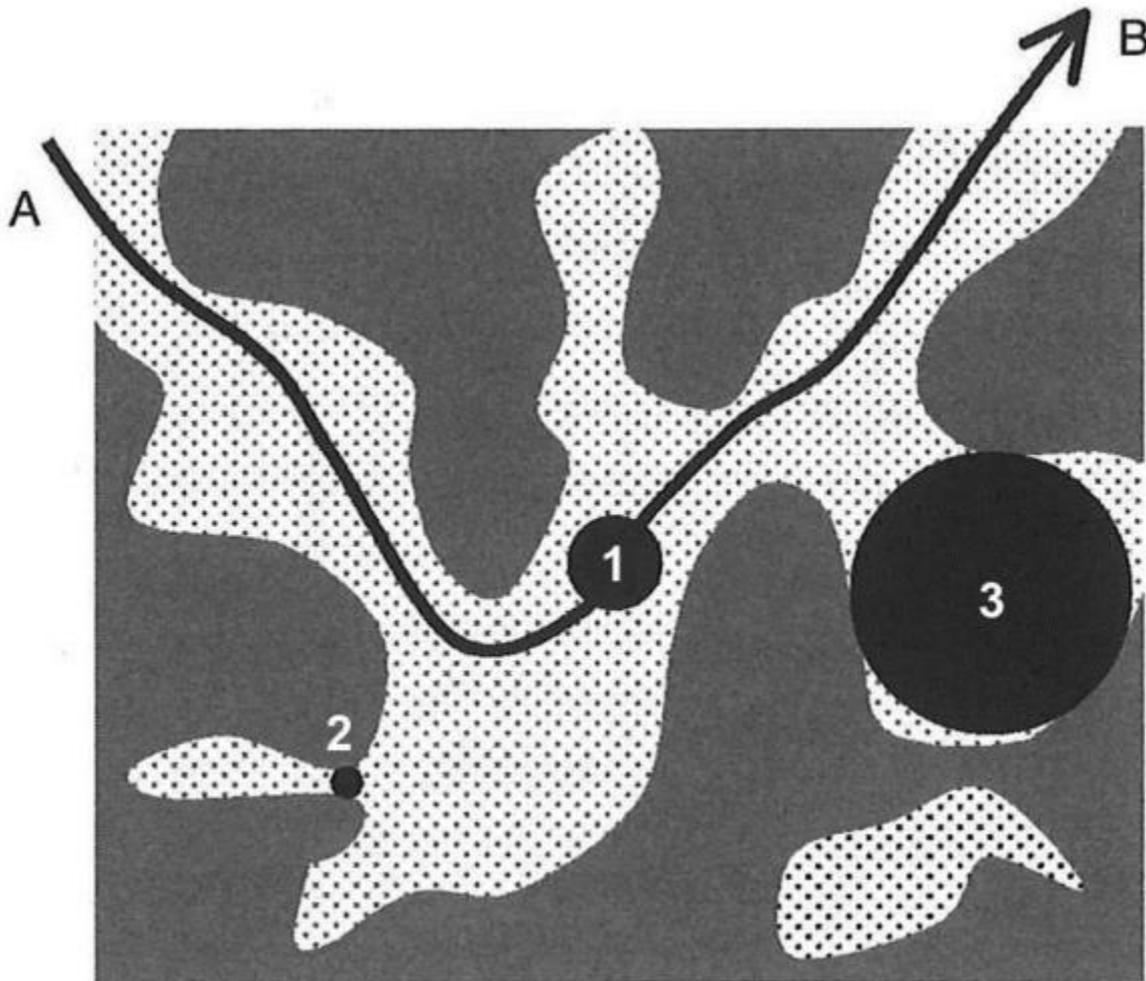
Figure 10 Graphic image of a porous material showing tortuosity of a path AB: the superimposed three black spheres indicate the minimum pore width on path AB (sphere 1) and the minimum and maximum pore widths in the shown pore structure (spheres 2 and 3 respectively). (Hall and Hoff, 2012, p.25, fig. 1.10 / Image © Spon Press)
