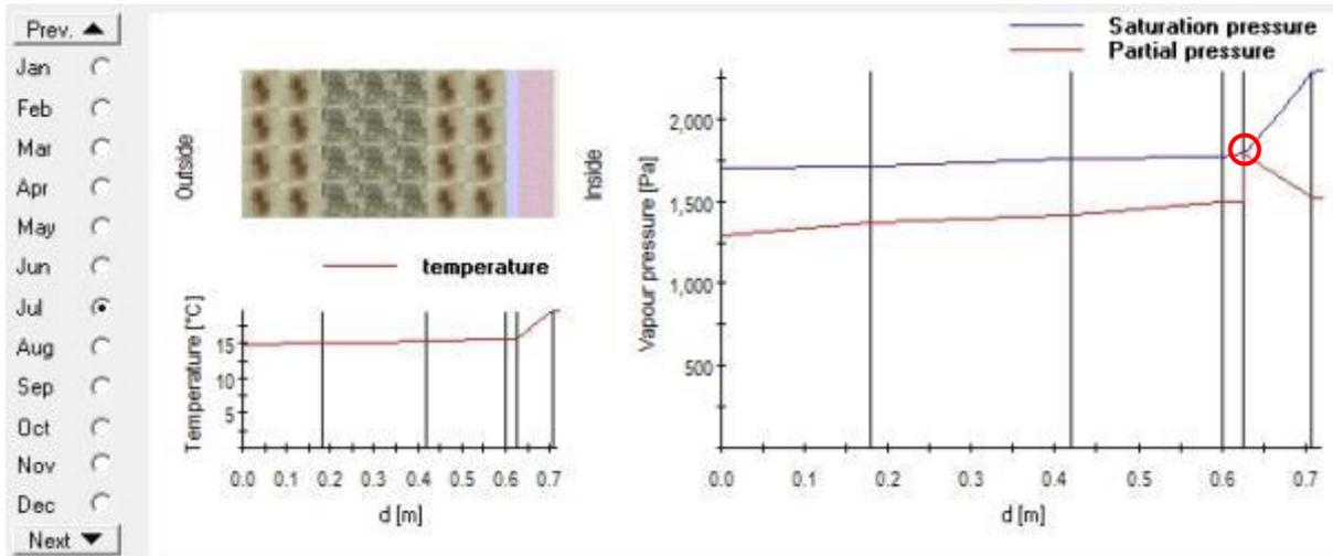
Figure 86 A partial screen shot from BuildDesk U showing the outputs of the July calculations of scenario 3.2.2 graphically, with the point of condensation circled
