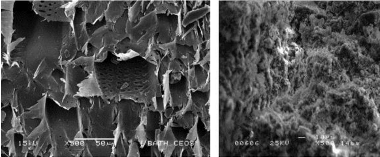
Figure 6 Scanning electron microscope photograph of hemp shiv fibres (left photo) and lime plaster (right photo), both at 250 x magnification. (Image © Mike Lawrence / University of Bath)
