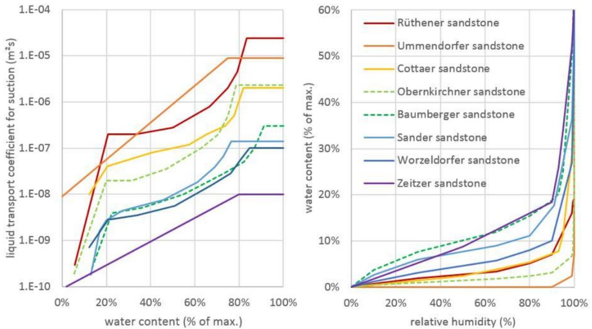
Figure 71 Capillary liquid transport (left) and moisture storage functions (right) of all German sandstones listed in the WUFI database.
