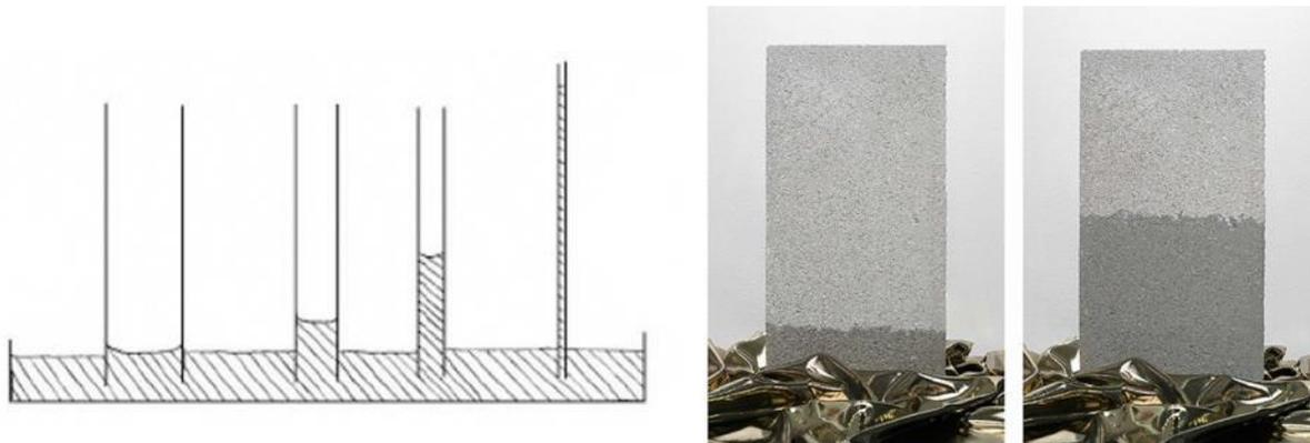
Figure 23 Liquid water risen vertically due capillary transport, illustrated graphically (left) and with two photographs showing rising water transport in a concrete block over time (right). (Left image: Torracca, 2009, fig. 3.17 / Image © The J. Paul Getty Trust) (Right image: Image © [APN MJM CC BY-SA 3.0](#))
