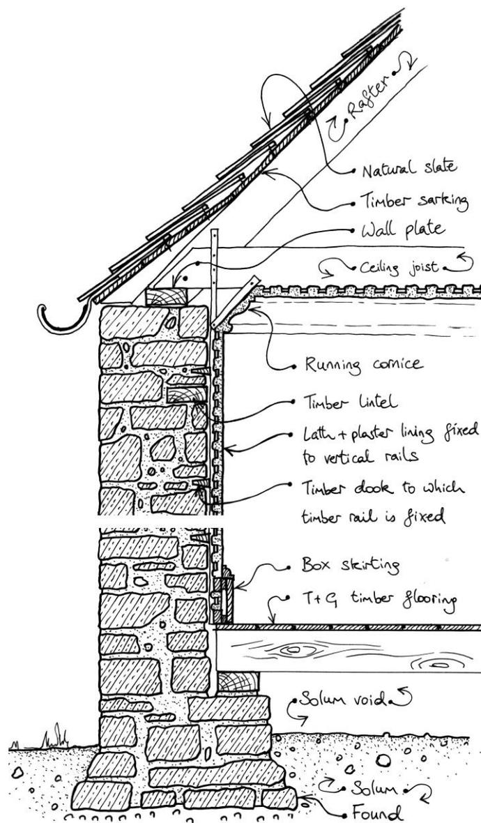
Figure 29 Cross sections through walls of traditional construction (left) and non-traditional construction (right)
