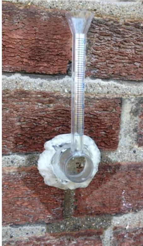
Figure 98 Karsten tube fitted to the surface of mortar joint in brick masonry
