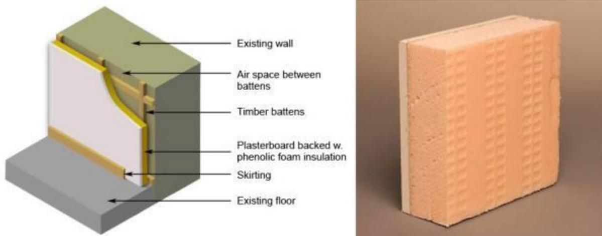
Figure 55 Phenolic foam insulation bonded to foil-backed plasterboard is fixed to timber studwork, leaving air cavities in between the studs and between insulation and masonry.
