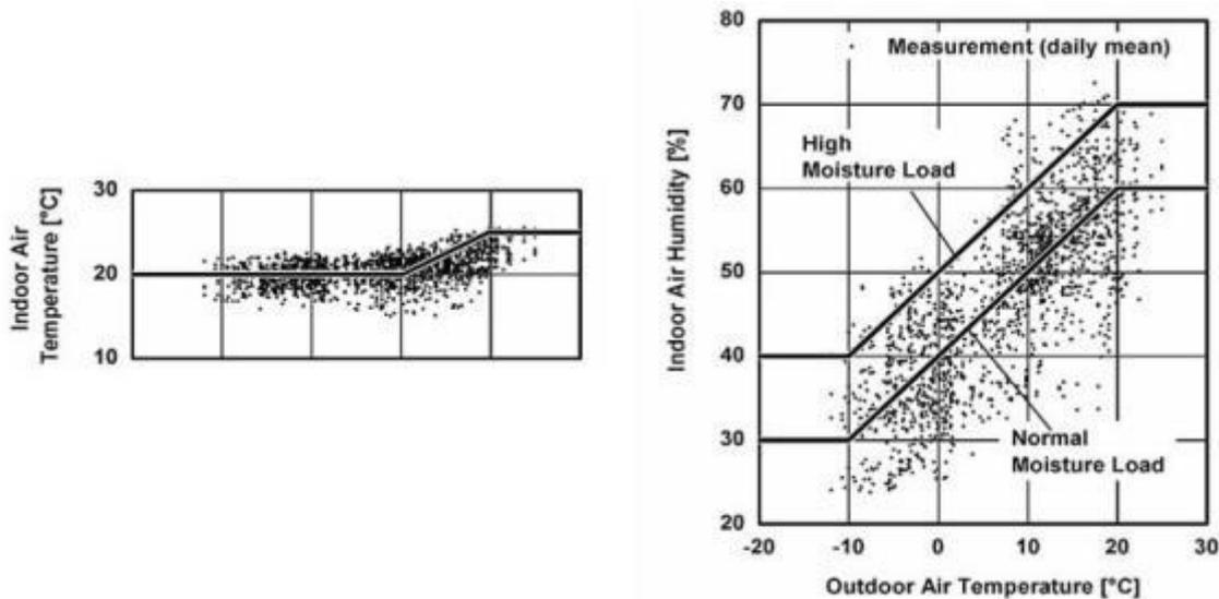
Figure 66 Correlation between indoor humidity and indoor and outdoor temperatures for simulation in accordance with *BS EN 15026:2007*
