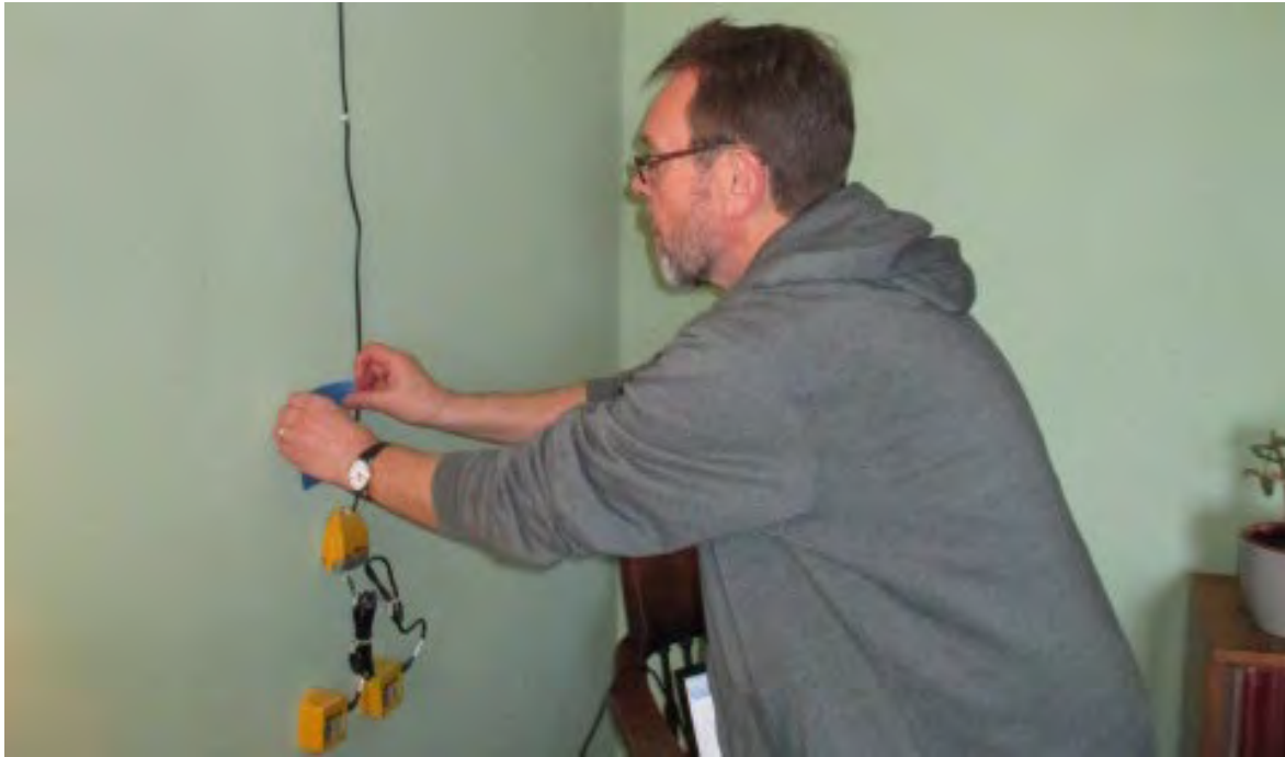
Figure 3. Installation of one of the heat flux plates.
