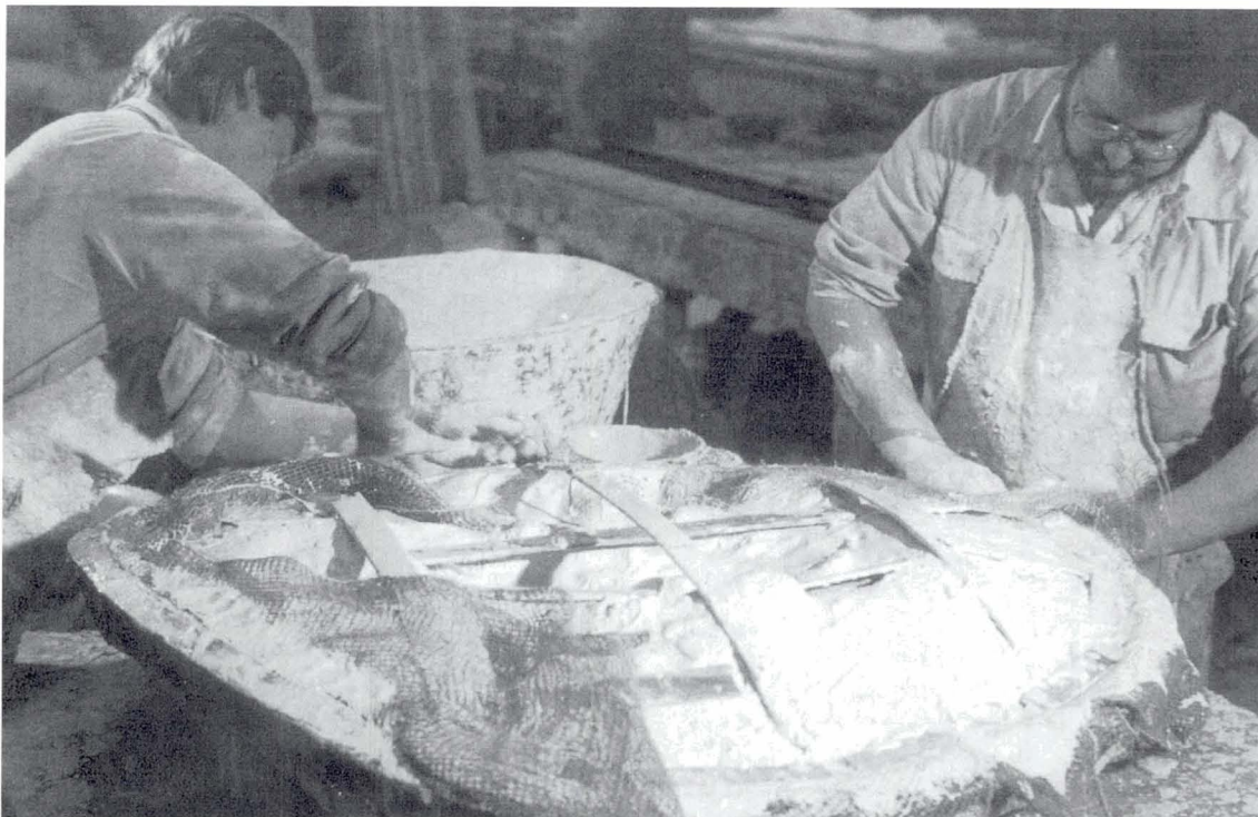
9. Fibrous plaster casting, at Chatelherault, 1984/5
