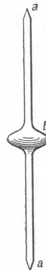
FIG. 15. a, Cutting edges of the jumper. b, Iron ball welded to the rod. Length of rod, 4 ft. 6 ins. to 5 ft. 6 ins.
