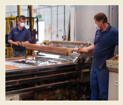
Fig. 4: The manufacture of sand cast lead sheet.
