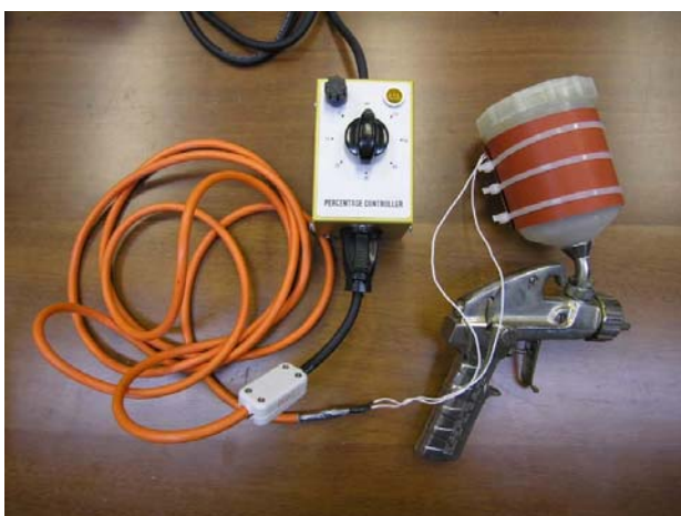
Illus. 12 Converted spray gun for cyclododecane
