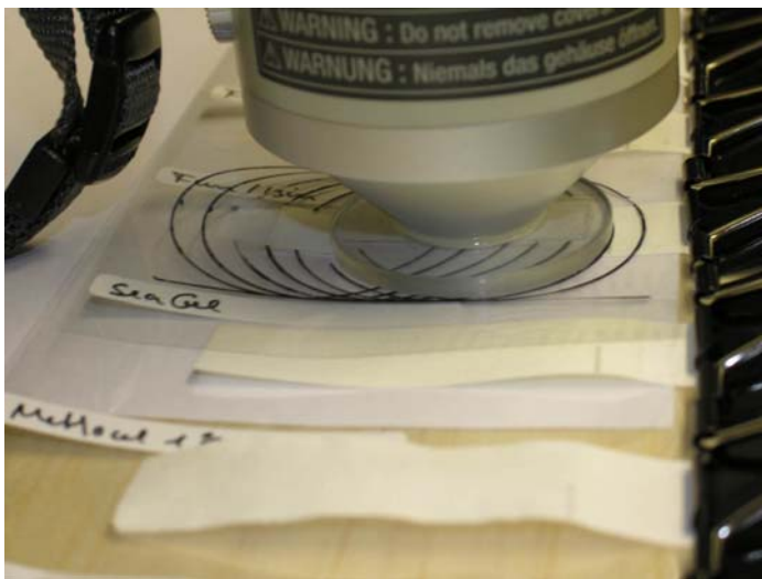
Illus. 20 With help of a template the colorimeter could be placed onto the same spots during repeated measurements
