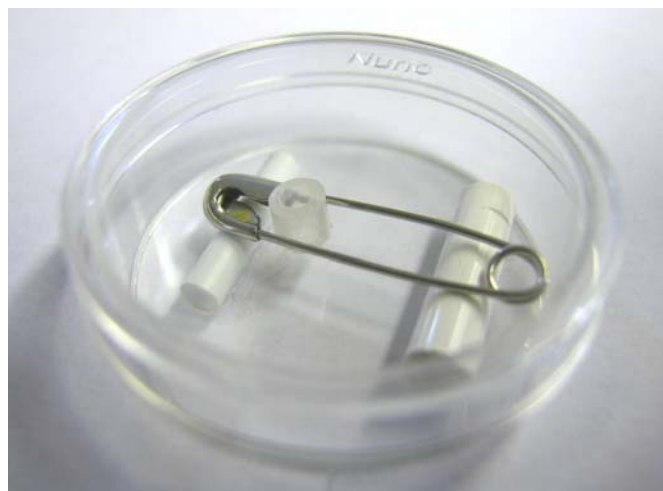
Illus. 39 Adapted container for swelling tests. The safety pin presses the two halves of a cut polypropylene tube together, which in turn hold the adhesive film in cross-section under the microscope.
