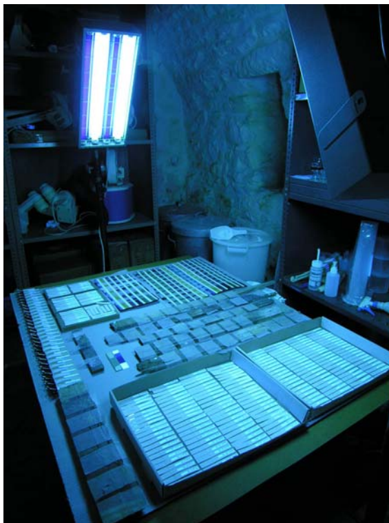
Illus. 19 The UV-ageing 'box' during the accelerated ageing in a lightless storage room
