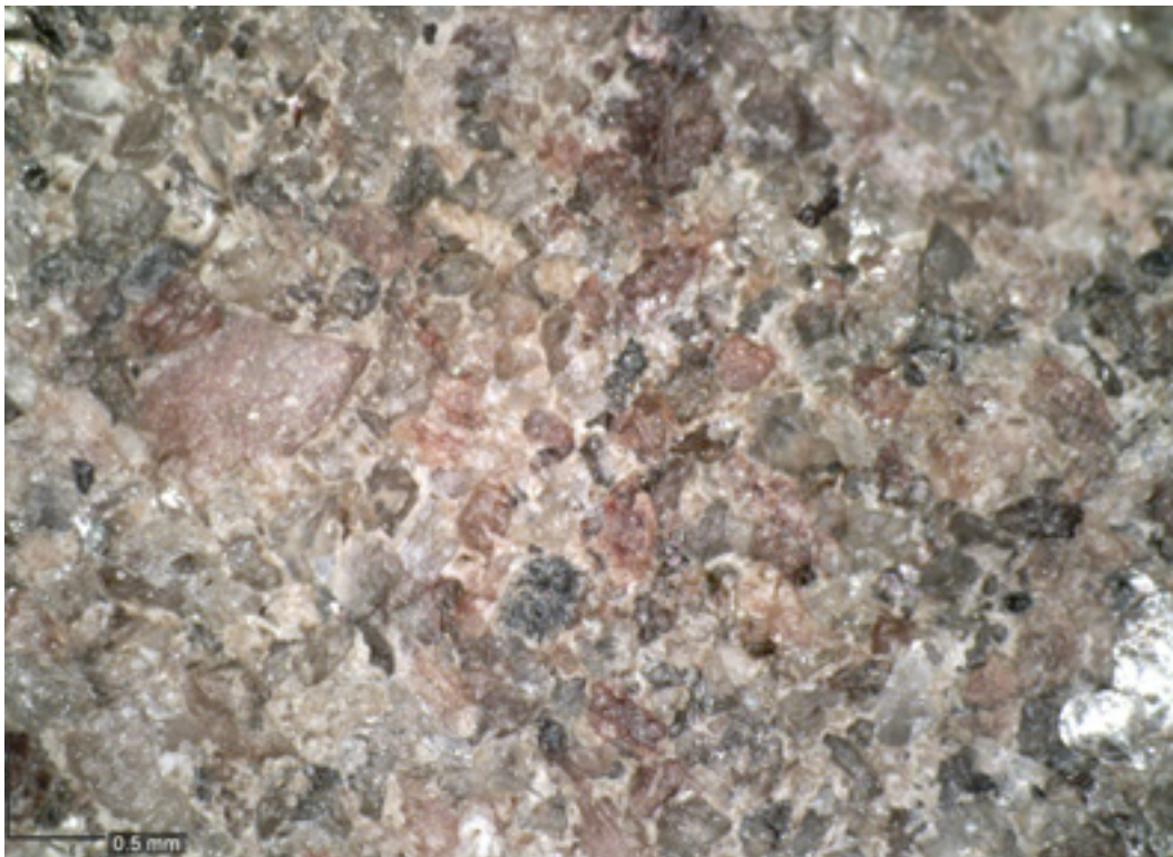
Fig 6. Difference in appearance between dark 'heart' shaped patch and an area of unstained stone on the top surface of the Stone of Destiny. Above: Sample area 1160 – dark surface staining on grains. Below: Sample area 1169 – clean open mineral texture on an adjacent area of non-stained stone.
