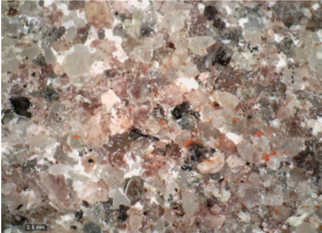
Fig 12. Sample analysis area 487 showing an accumulation of deposited red material (centre right of image).
