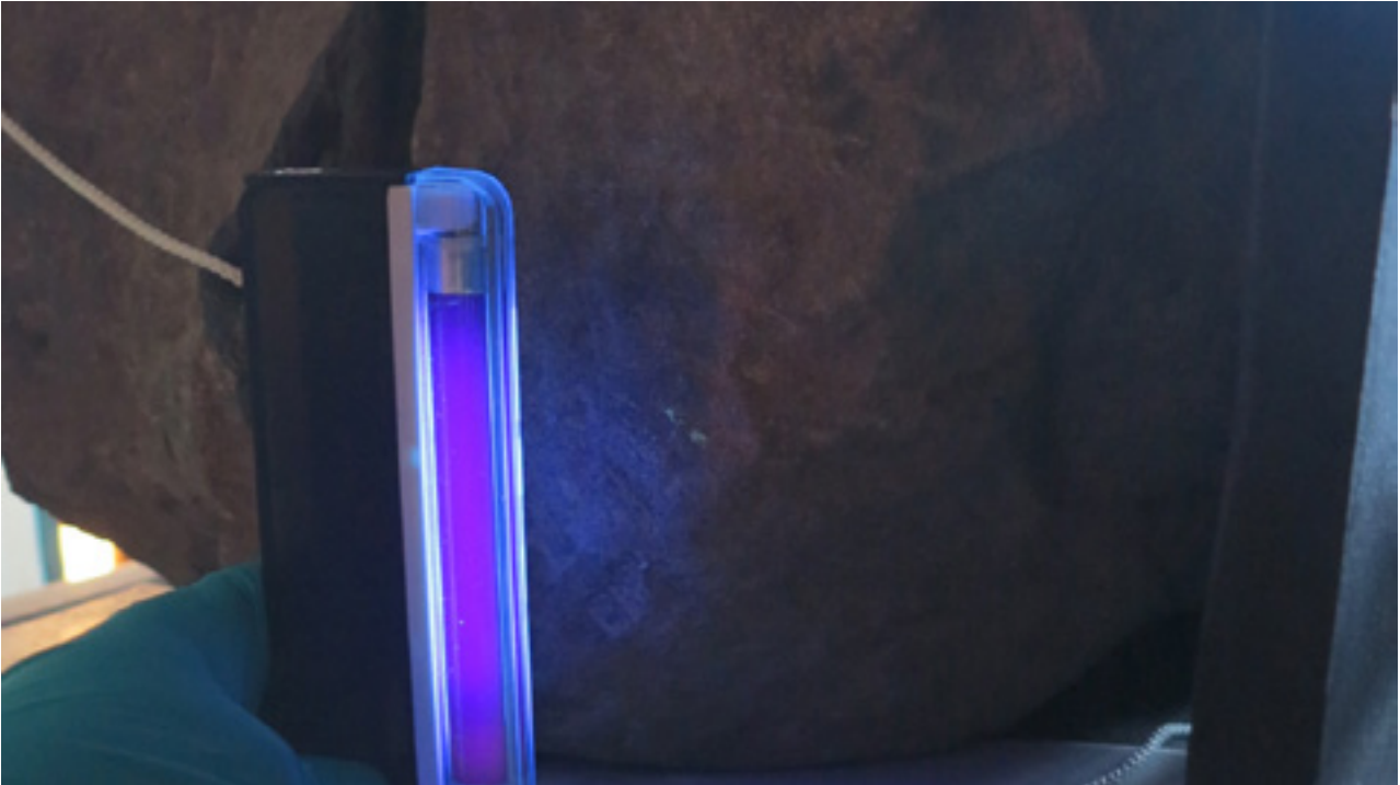
Fig 38. The sinister end face under UV light and the three fluorescing areas visible (2023).
