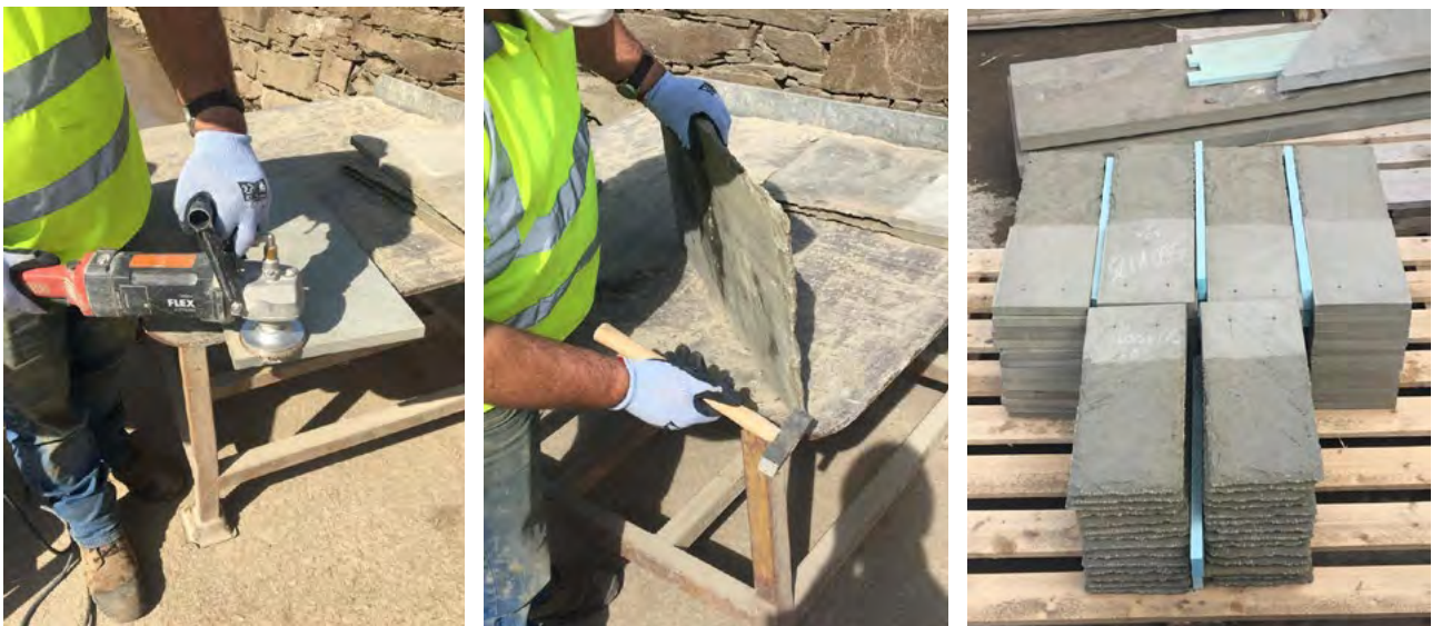
Figure 45a, b and c: Flagstone being hand finished at Pitairlie Quarry by Denfind Stone, and as delivered. © Douglas Binnie.
