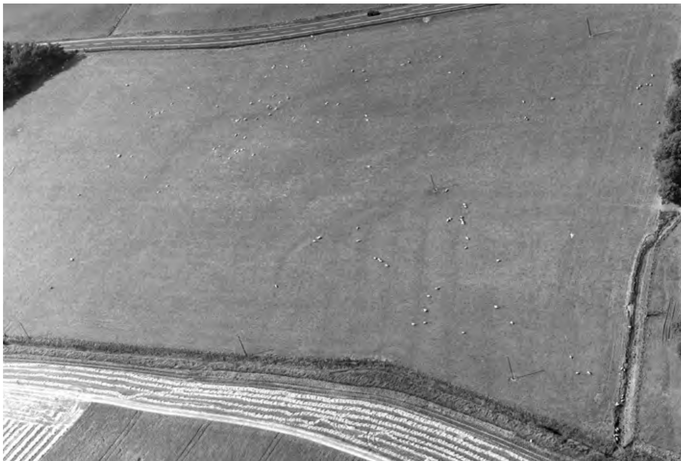
Fig 80 The furrows and ridges of this water meadow are fed by a header drain that curves around the end. Townhead Farm, Lanarkshire. SC505315.
