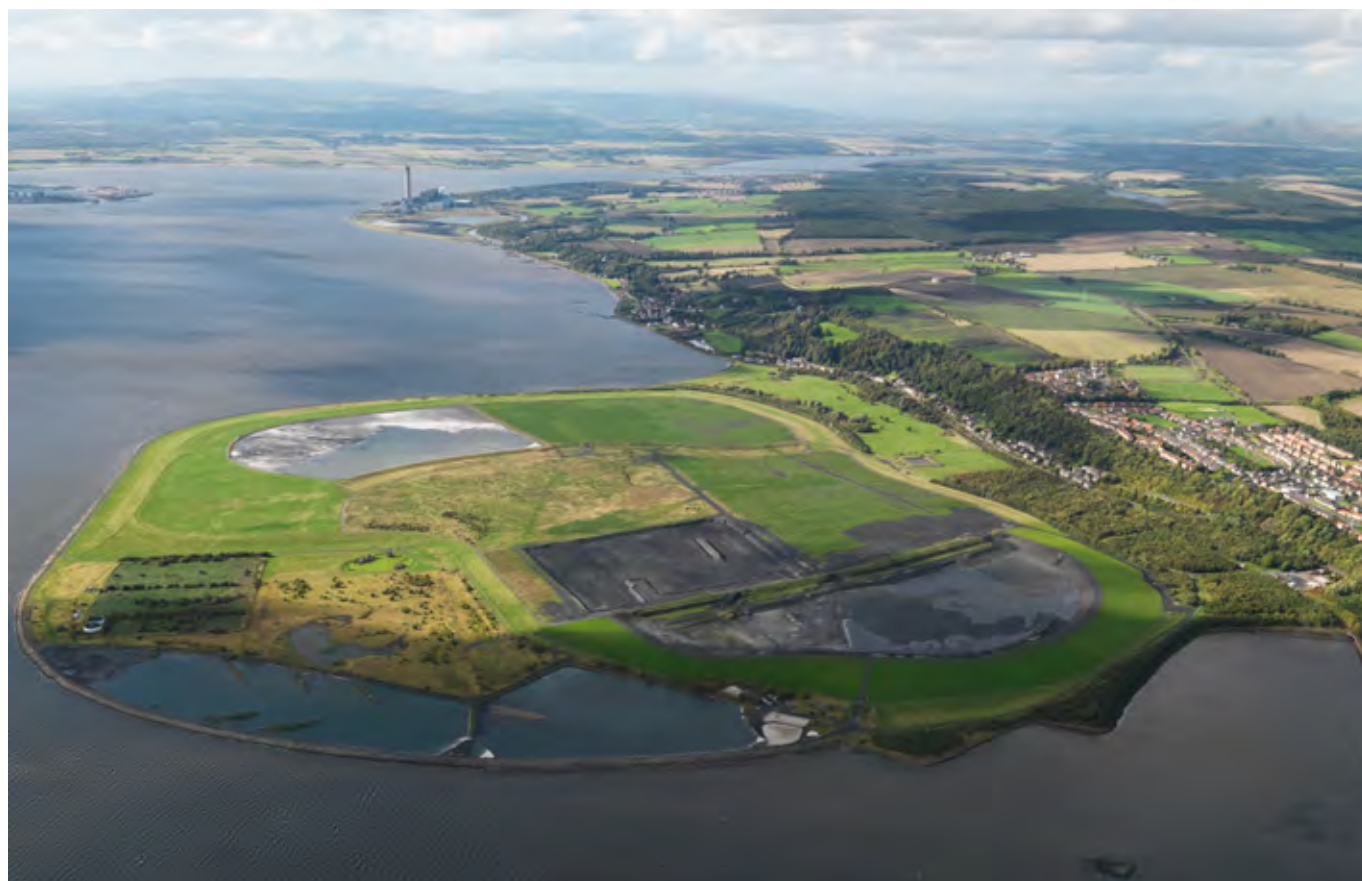
Fig 67 Longannet power station, with its chimney visible in the background, produced huge quantities of ash that was stored in the lagoon at Preston Island. DPO88447.
