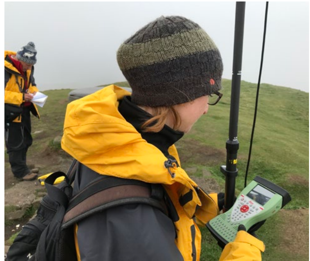
Using a differential GPS to accurately map the archaeology of East Lomond Hill, Fife.
