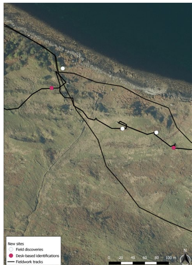
The GPS-recorded tracks of routes walked during fieldwork shown against an orthophotograph. In this case the route taken was designed to check selected desk-based identifications and also to explore the landscape for previously unrecognised sites. Aerial imagery © Getmapping plc
