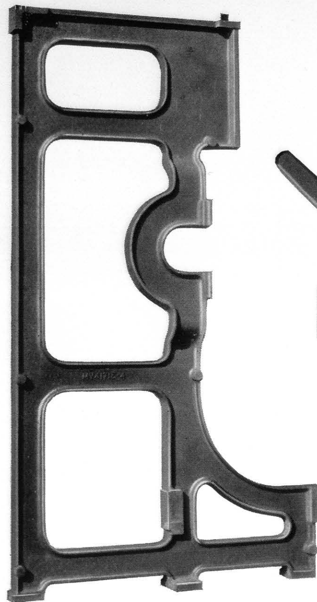
C.I. Machine Frame 6' 4" High x 3' 8" Wide Overall x 2" Deep
