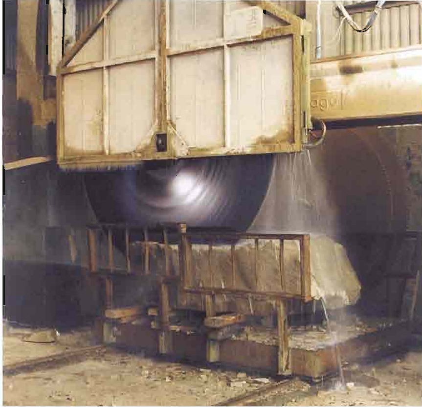
Primary sawing process: circular diamond-tipped blade (above) and monoblade (below) saws in use
