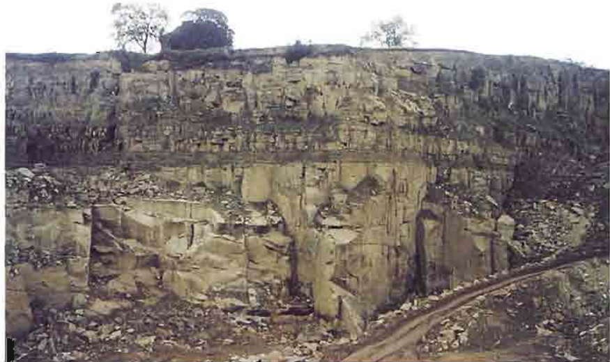
English quarries also supply stone to the Scottish market. Stanton Moor is a popular choice because of its similar colouring to that of many existing buildings in Scotland's main cities.
