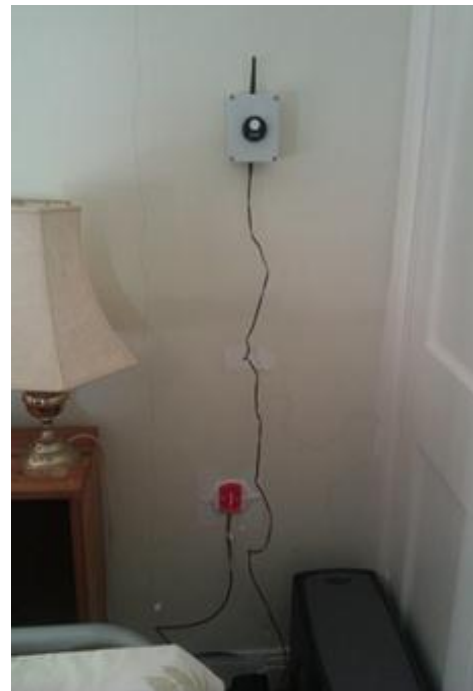
Fig. 7 Monitoring equipment installed at Scotstarvit Tower Cottage. Internal CO 2 , temperature and RH sensors in living room. Note: red heat flux plate at base of this picture is not associated with this study.
