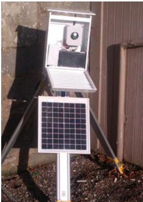
Fig. 6 Monitoring equipment installed at Scotstarvit Tower Cottage. External CO 2 , temperature and RH sensors (shown with the screen open).
