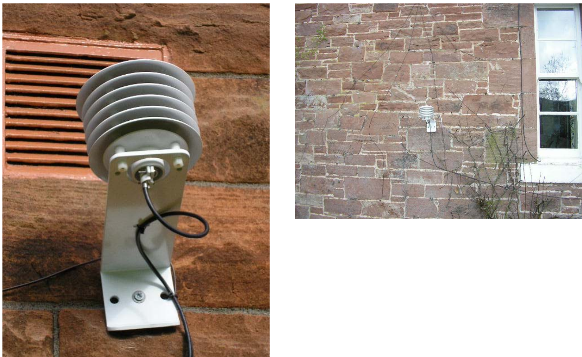
Figure 3: Mounting of shielded external temperature sensor
