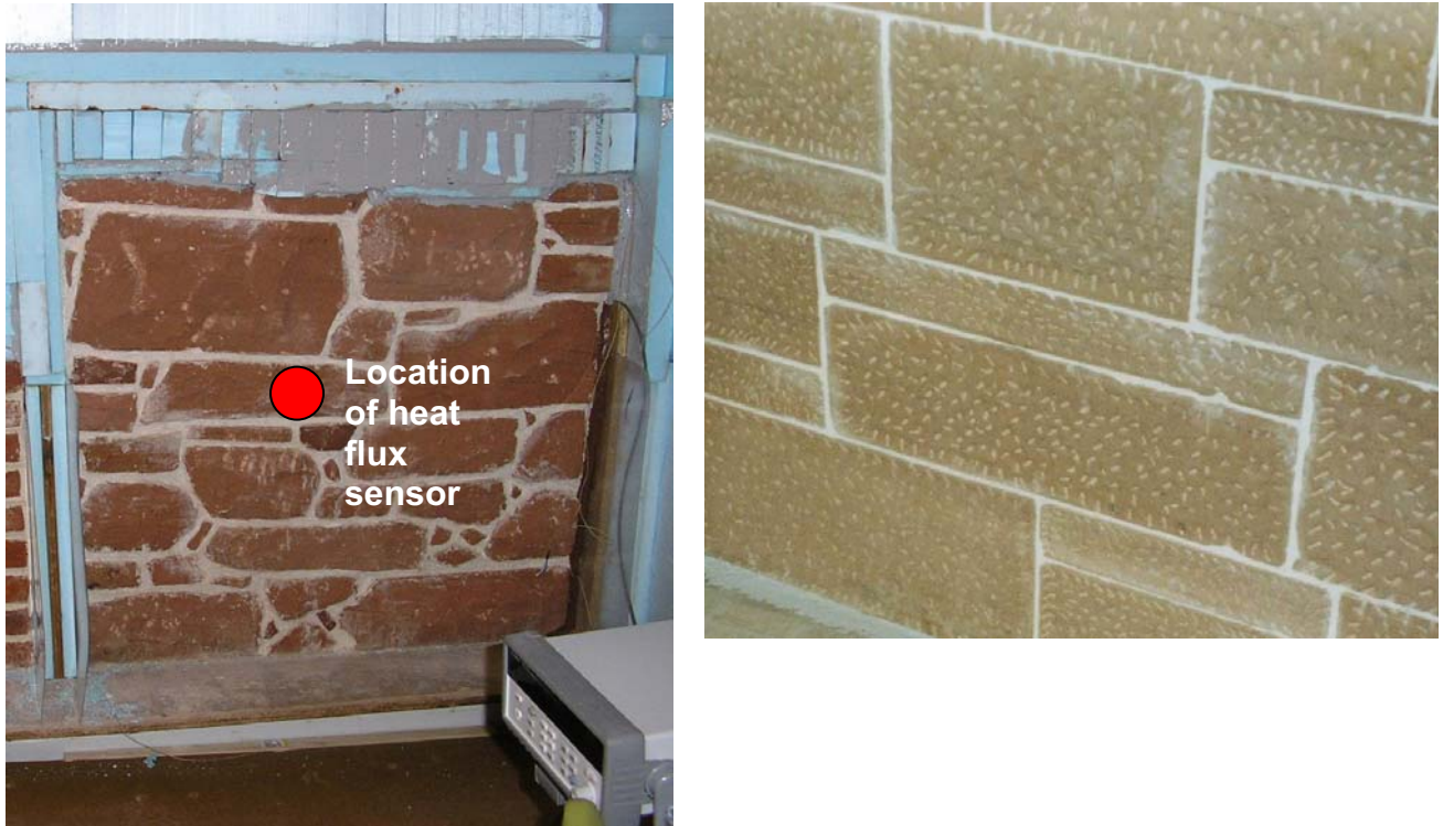
Figure 15: Locharbriggs sandstone wall in test chamber. Left: internal rubble face; right: Ashlar external face.
