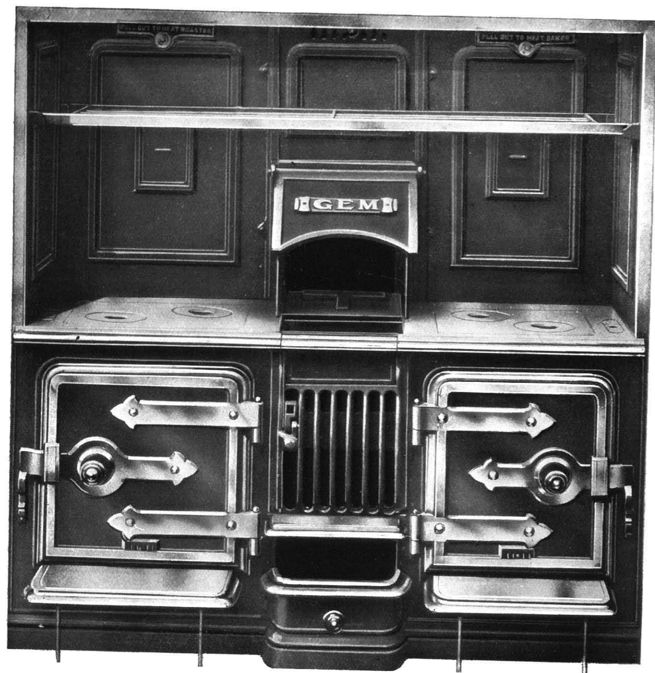
No. 208 "GEM" RANGE, double oven, close and open fire, strong sheet-iron ovens full depth of hobs, bright bracket shelves with wrot.-iron stay rods. "Radial" rising fire, with fall bar, lift-off bracket shelf and ashpan, open and close fire arrangement, sliding fire cover, full cast-iron covings, long rod oven dampers with inscription plates, wrot.-iron plate rack with polished front. Sheet-iron covering-in plate with sliding door. All mouldings and mountings bright.
