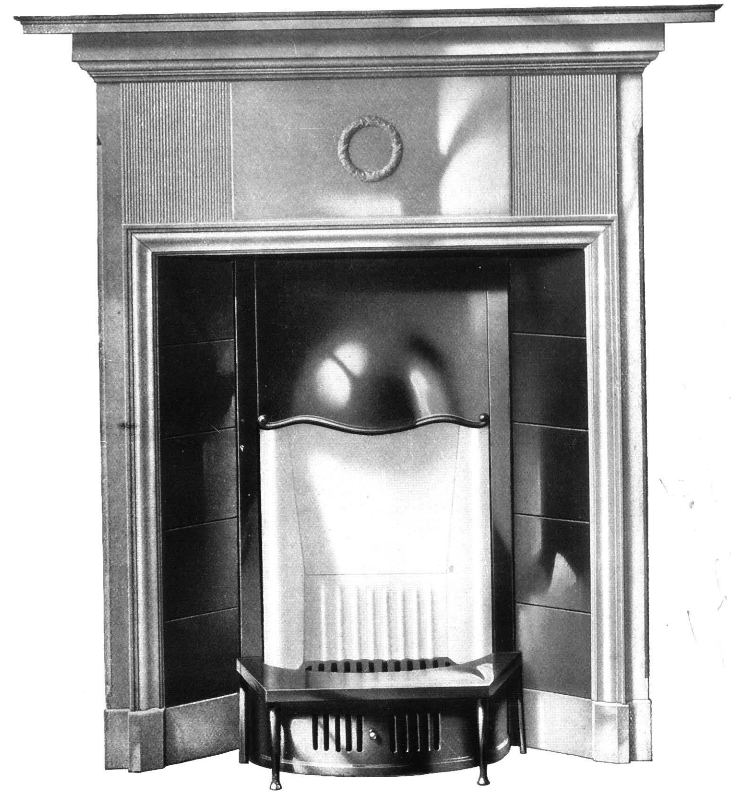
No. 788 TILE MANTEL GRATE, with single shelf, adjustable cast-iron canopy, sectional brick back, “ Alpha ” fire, with sliding draught regulator and No. 35 Trivet Hob. Prepared for Tiles.
