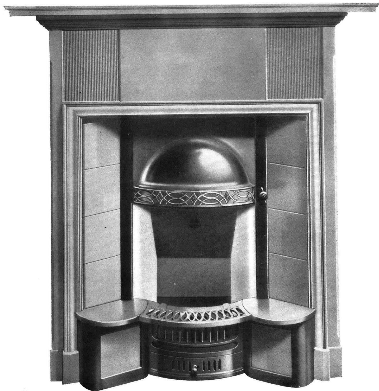
No. 827 HOB TILE MANTEL GRATE, with single shelf, adjustable cast-iron canopy, sectional brick, steel spindle bars, hook-on trivet and slow-combustion fret with sliding draught regulator, No. 2 self-contained cast-iron back and boiler flue. Prepared for tiles and high pressure boiler.
