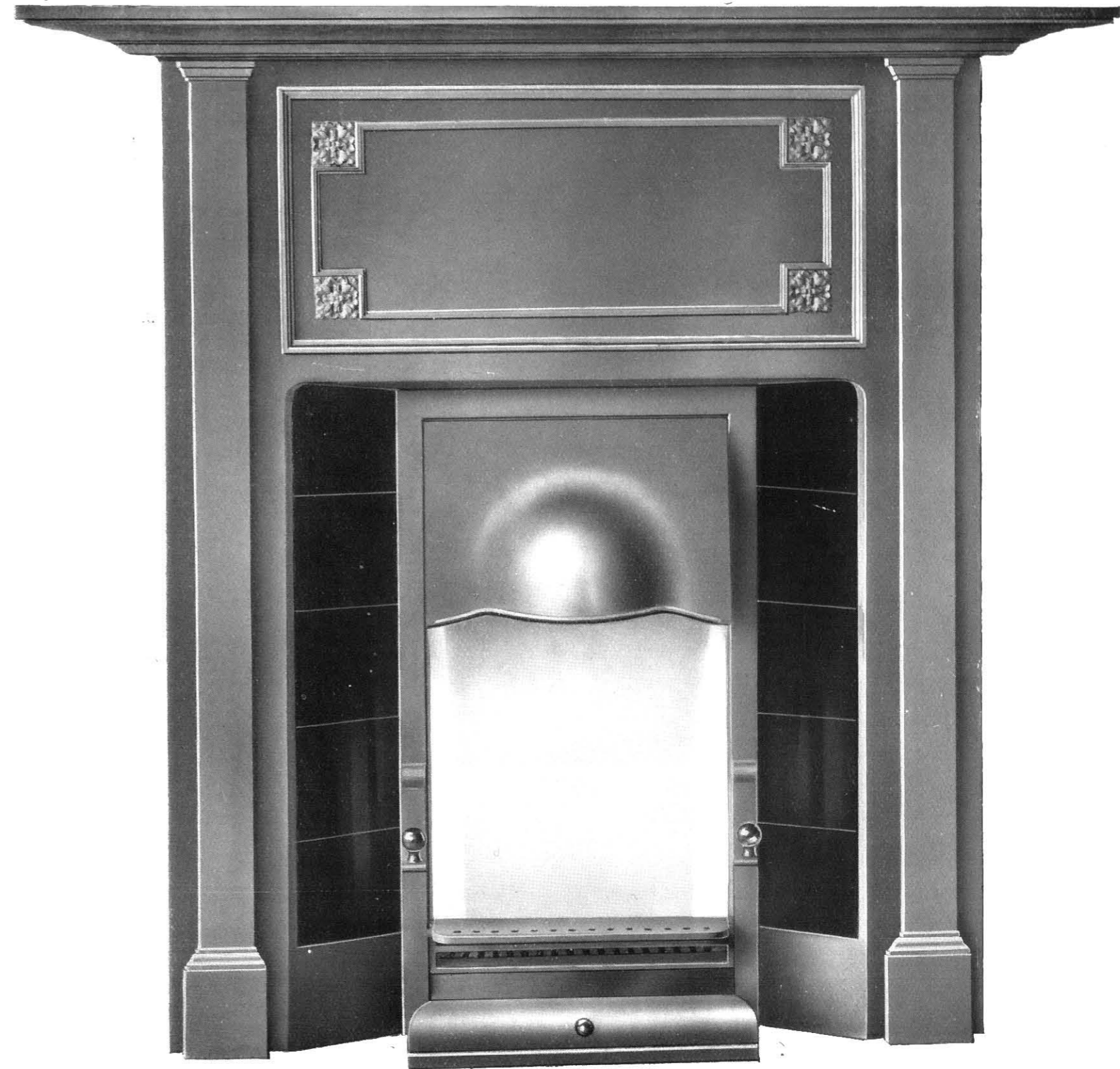
No. 741 TILE MANTEL GRATE, with double shelf and adjustable cast-iron canopy, N/C/ solid brick back, “ Solar ” fallbar fire, with brass or copper knobs, slow-combustion fret, prepared for tiles.
