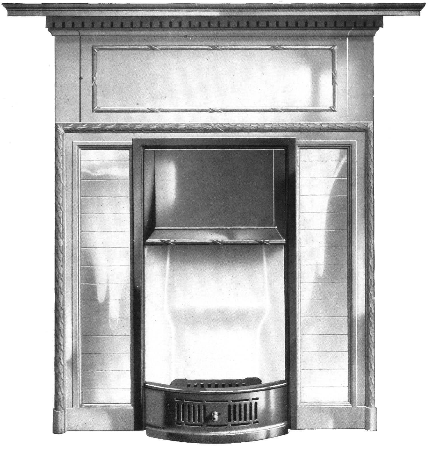
No. 794 TILE MANTEL GRATE, with single shelf, adjustable cast-iron canopy, W/S solid brick back with vent damper, “ Douglas ” fire with sliding draught regulator. Prepared for tiles.
