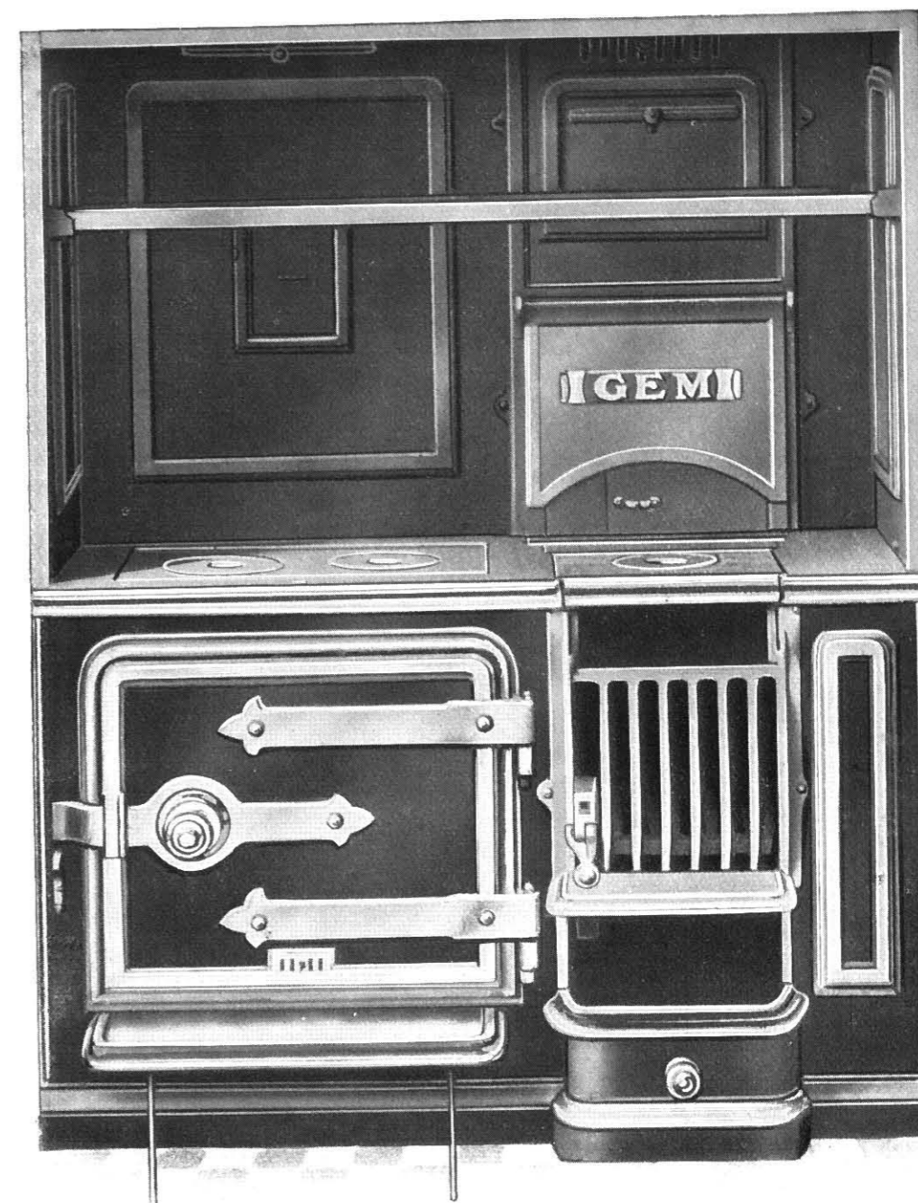
No. 207 "GEM" RANGE, combined open and close fire, with strong sheet-iron oven on right or left hand, bright bracket shelf with wrot.-iron stay rods, "Radial" rising fire, with fall bar, lift-off bracket shelf and ashpan, open and close fire arrangement, sliding fire cover, full cast-iron covings, wrot.-iron plate rack, sheet-iron covering-in plate with sliding door. All mouldings and mountings bright.
