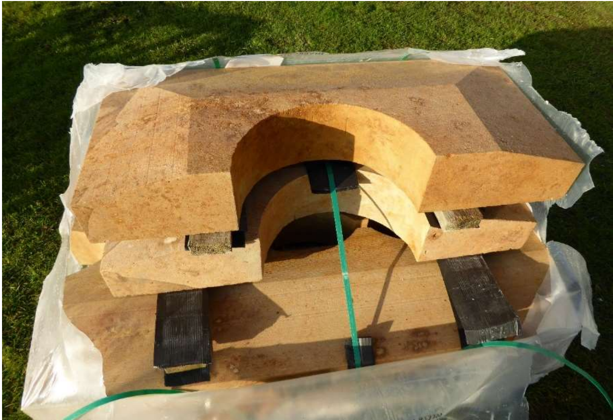
Figure 19: New stone chimney copes.
