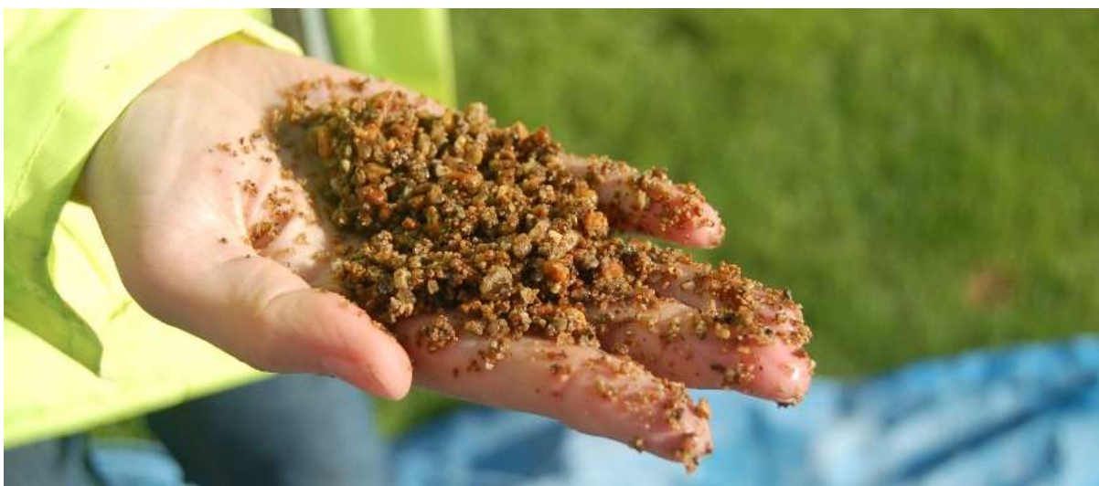
Figure 15: Sand and aggregate from the beach similar to that present in the original harl.
